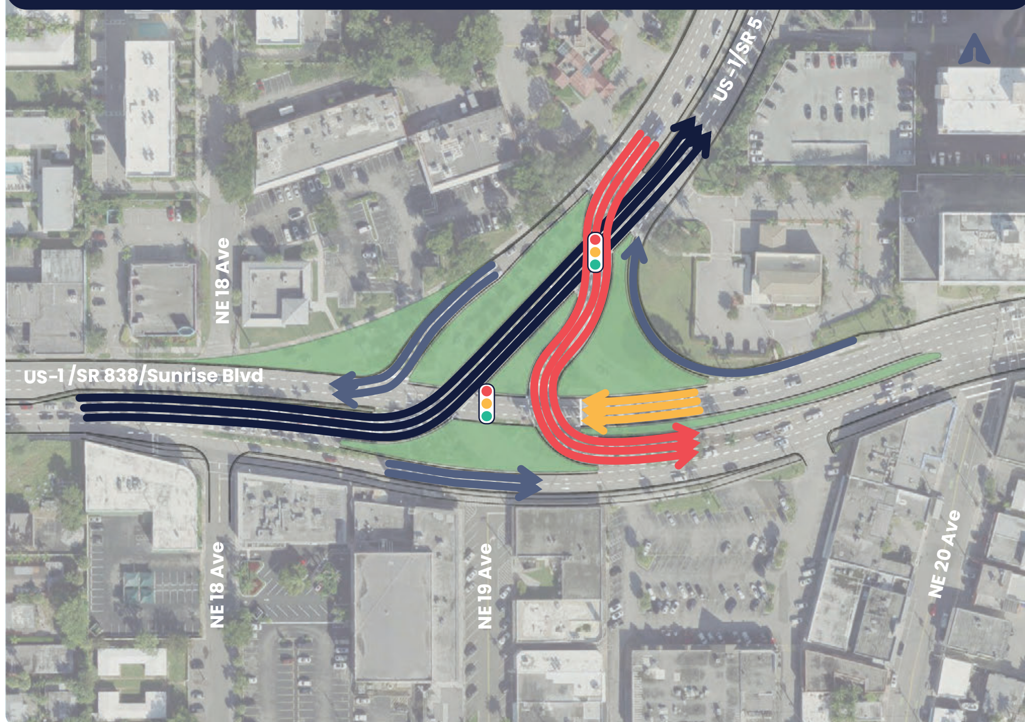
Concept 4 EB Upstream Triple Left Signalized At-Grade T with SB Displaced Left
