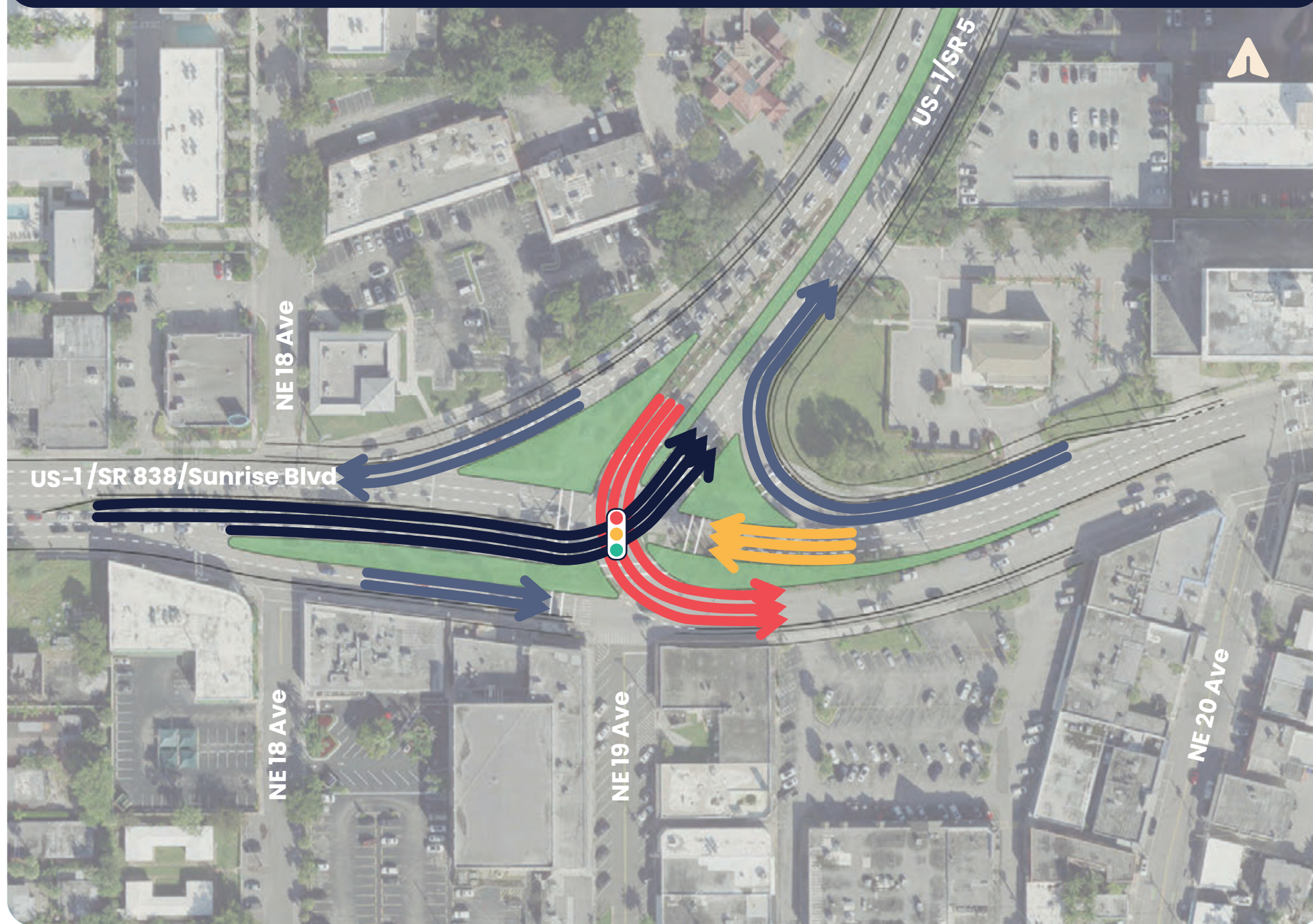
Concept 1 EB Triple Left Signalized At-Grade T
