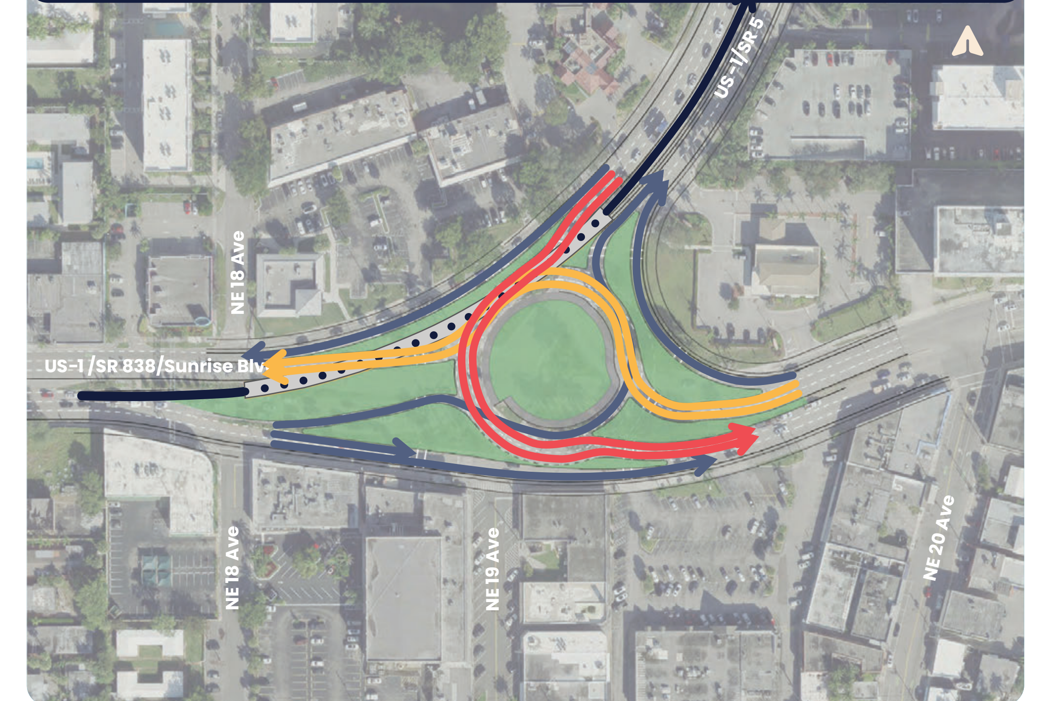
Concept 6 Multilane 3-leg Roundabout with EB Left Turn Compressed Underpass (underground vertical separation)
