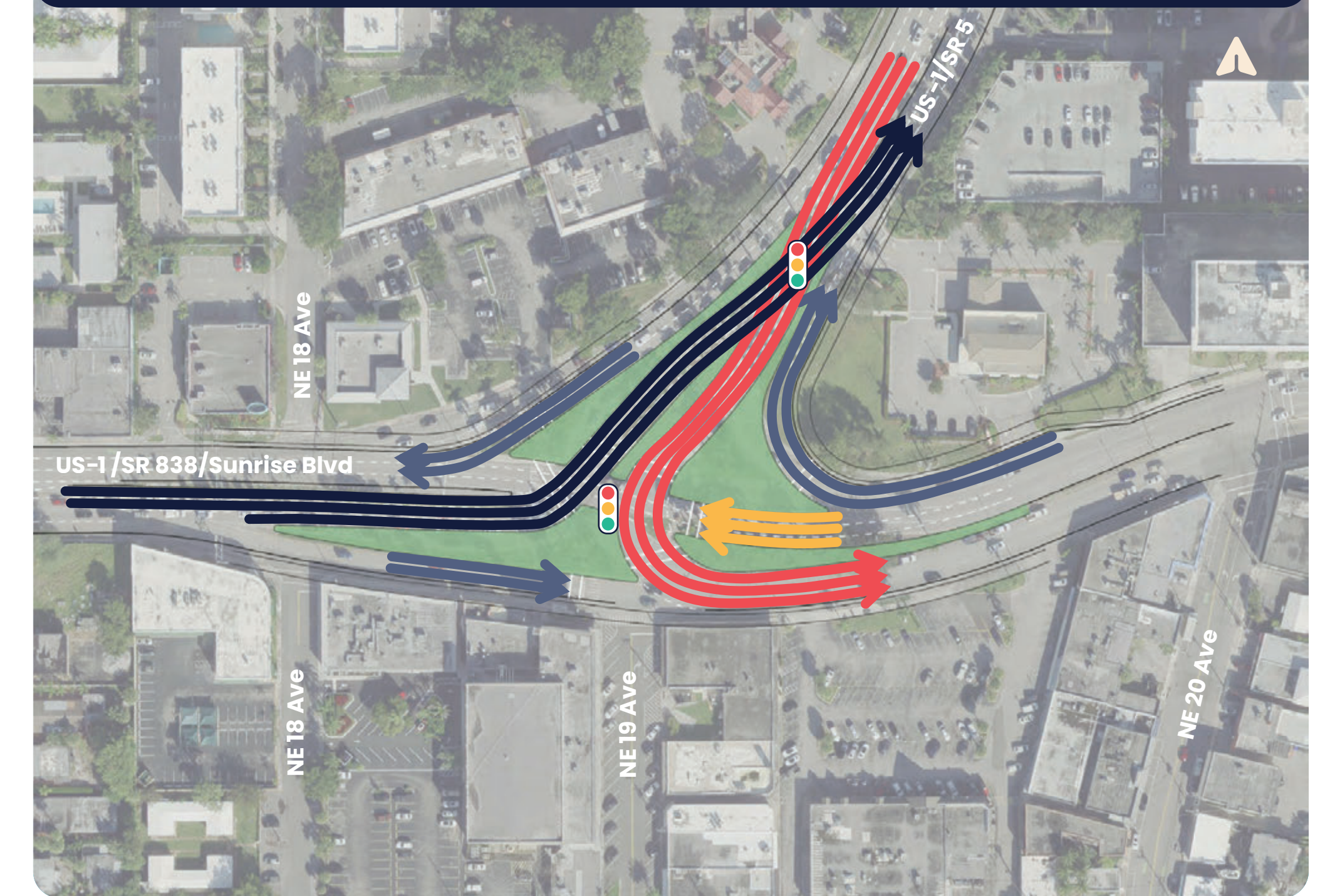
Concept 3 EB Upstream Triple Left Signalized At-Grade T with SB/NB Crossover
