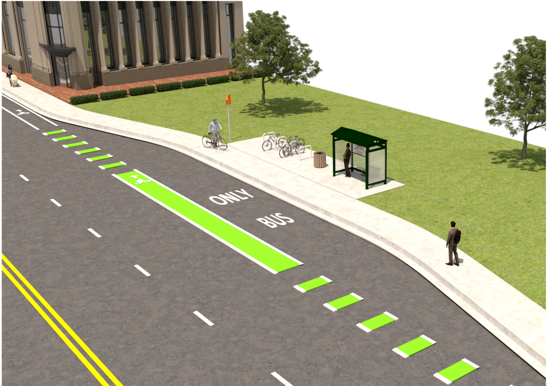
Figure D.2.2 | Enhanced bus stop.
