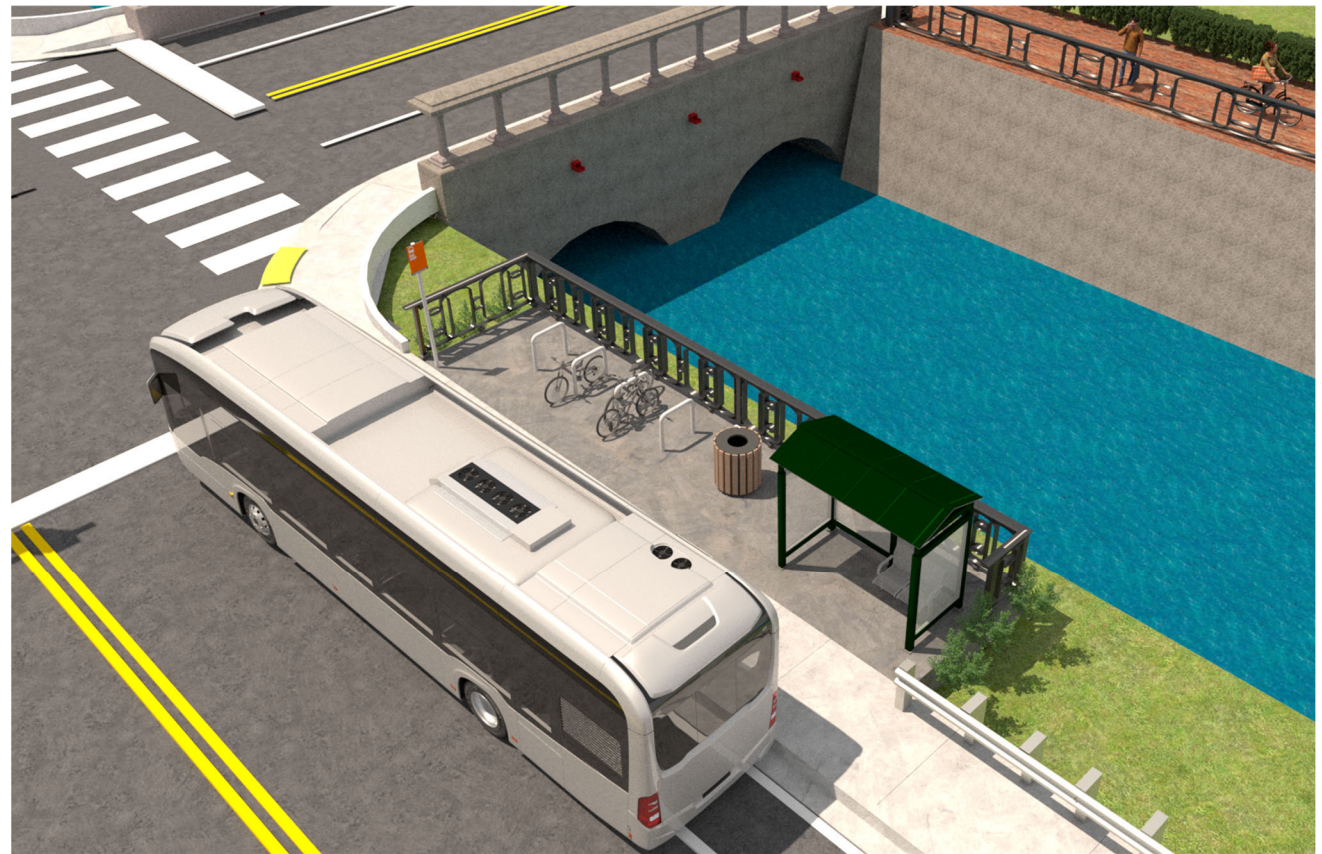
Figure 4.2.1 | Bus stop located near a canal and adjacent to a guardrail.
