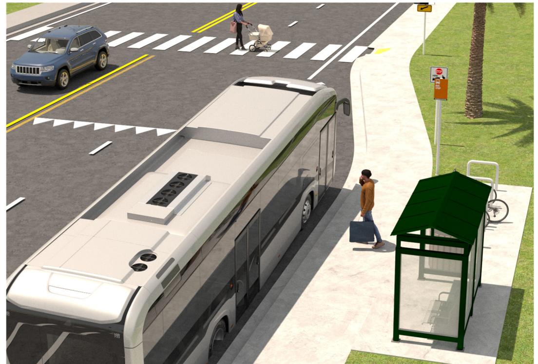
Figure 4.6.3 | Mid-block pedestrian crossing near a bus bay.
