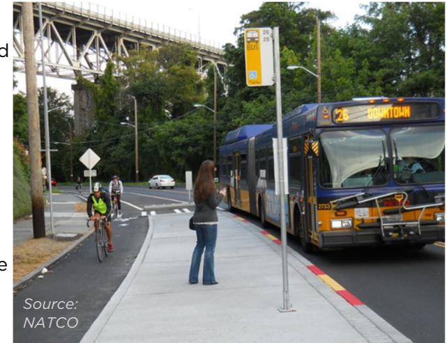
Figure 4.6.12 | Example of a boarding island.
