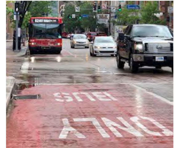
Figure 4.4.1 | Example of a curbside bus lane.
