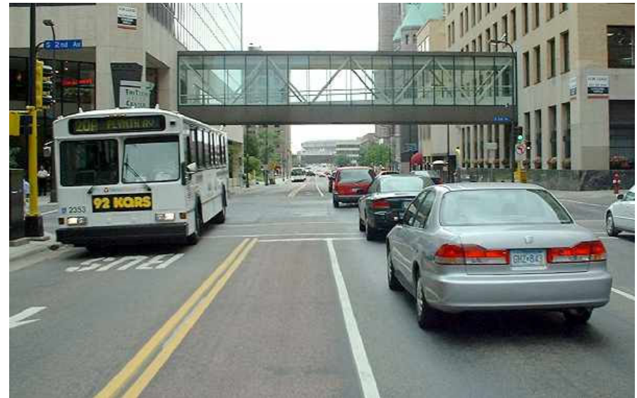
Figure 4.4.3 | Example of a contraflow bus lane on a one-way street.
