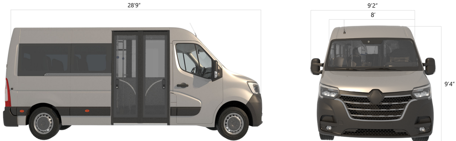
Figure 4.5.3 | On-demand or paratransit vehicle typical dimensions.
