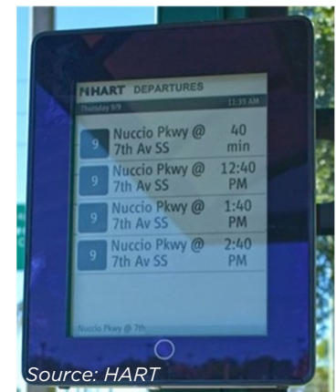
Source: HART Figure 3.9.2 | Digital ink display in Tampa, Florida.
