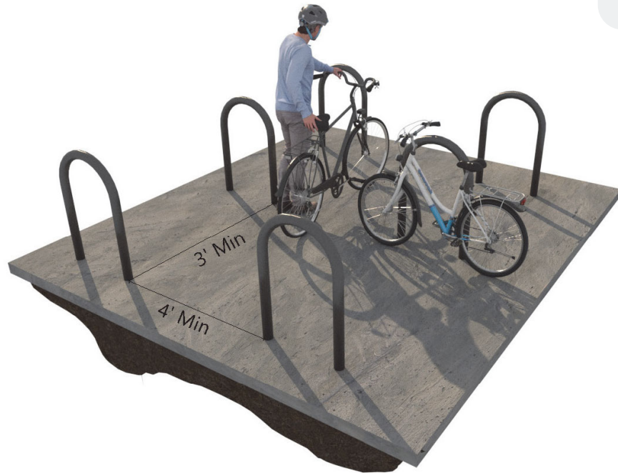
Figure 3.5.2 | Dimensions for accessible bicycle rack placement.
