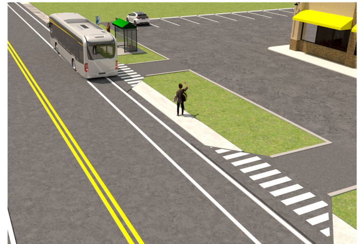
Figure 4.2.3 | Acceptable bus stop placement near two driveways.
