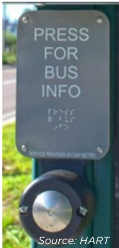
Figure 3.8.4 | Pushbutton-activated system at a bus stop.
