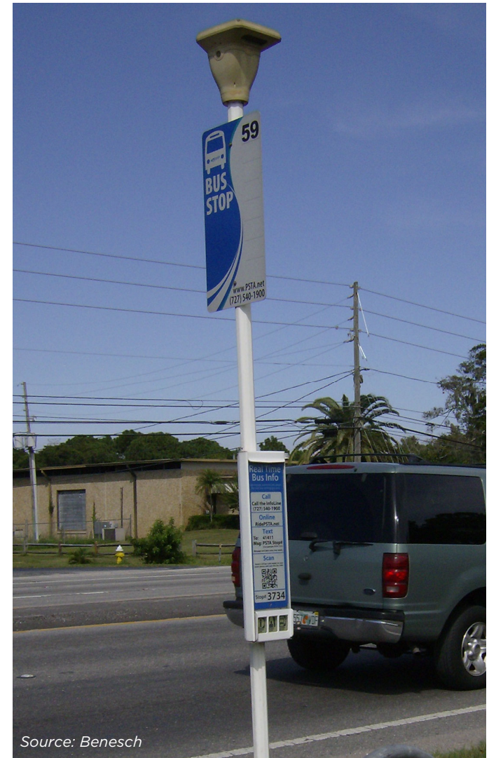
Figure 3.10.1 | Solar-powered bus stop sign with bus signaling and lighting capabilities, Pinellas County, Florida.
