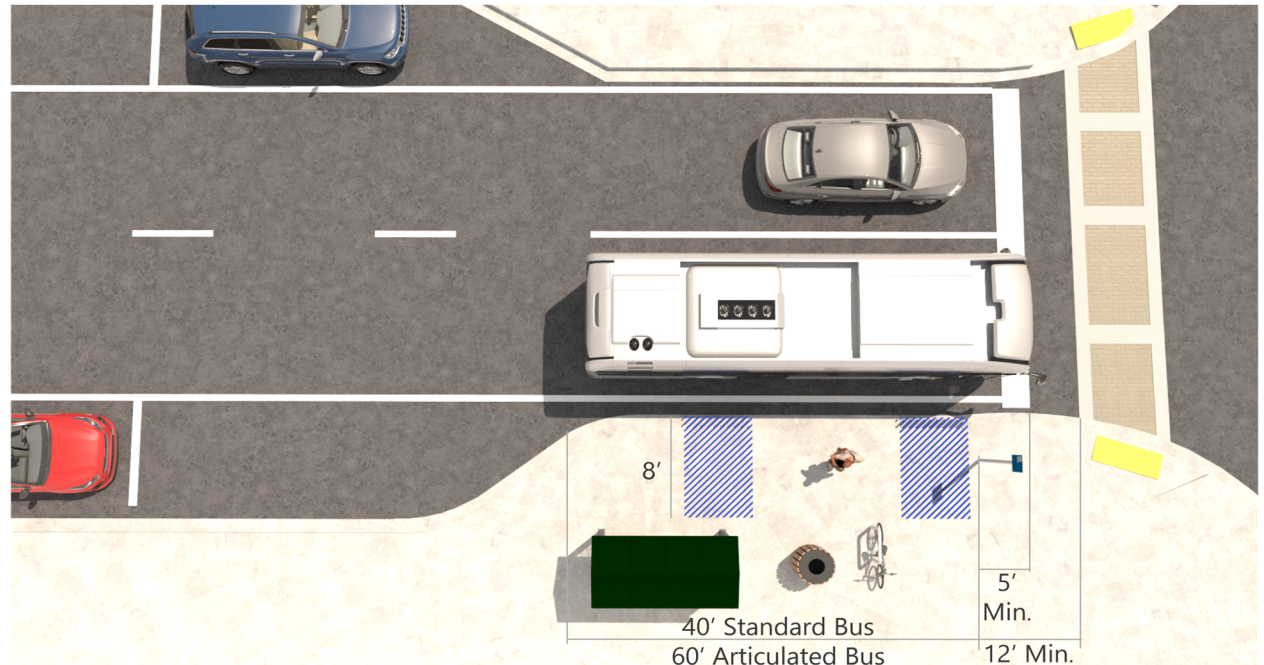
Figure 4.3.3 | Dimensions of a near-side bus bulb bus stop.
