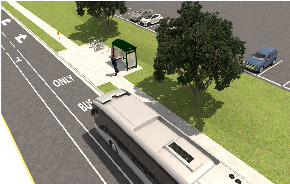
Figure 4.3.8 | Example of an open Bus Bay.
