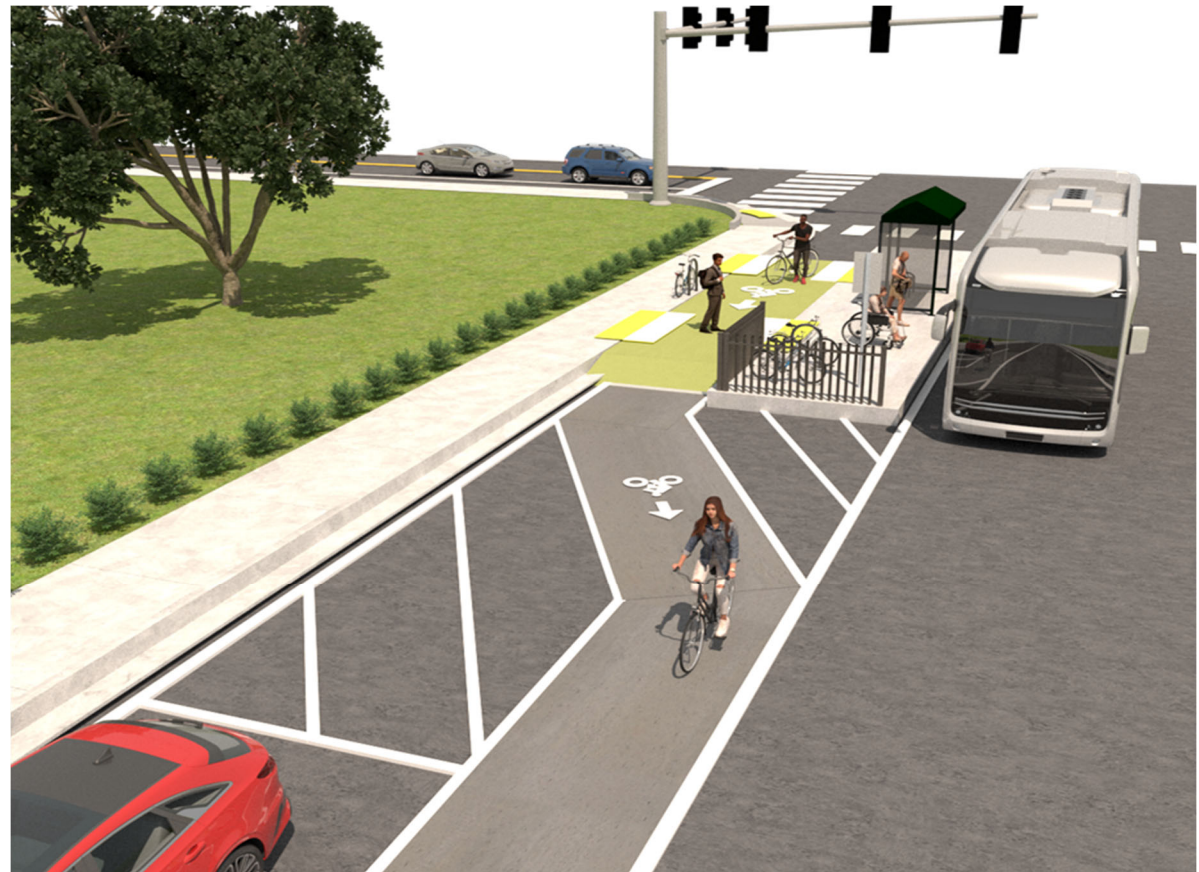
Figure 4.3.4 | Example of boarding island/floating bus stop.
