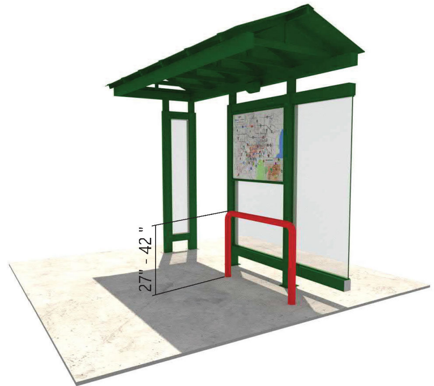
Figure 3.8.1 | Dimensions of a bus stop leaning rail.
