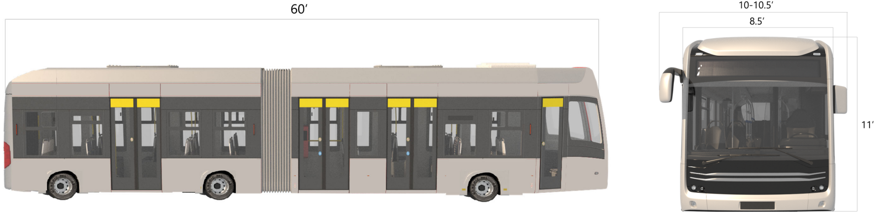
Figure 4.5.2 | Articulated bus typical dimensions.
