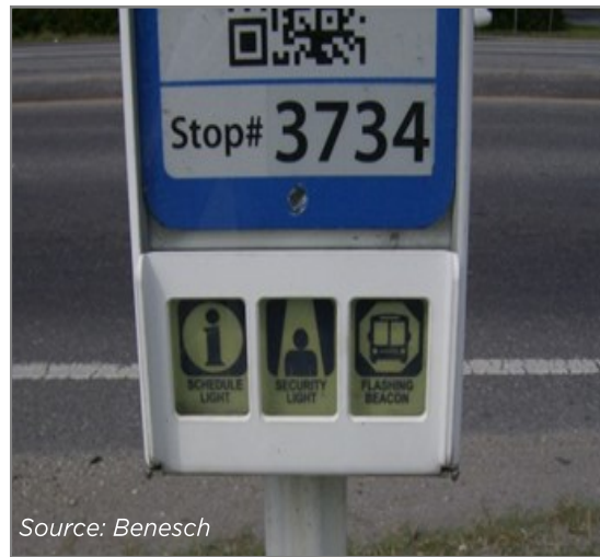
Source: Benesch Figure 3.10.3 | Details of a solar-powered bus stop signpost with bus flagging capability and security lighting, Pinellas County, Florida.
