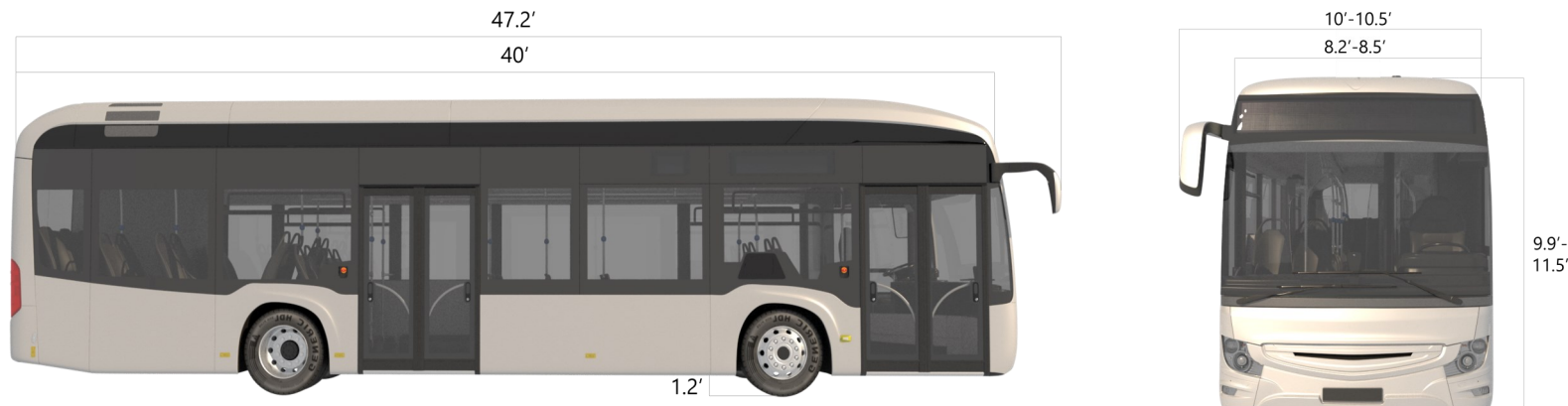
Figure 4.5.1 | Standard fixed-route bus typical dimensions.
