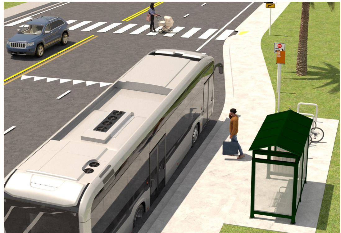
Figure 4.6.3 | Mid-block pedestrian crossing near a bus bay.
