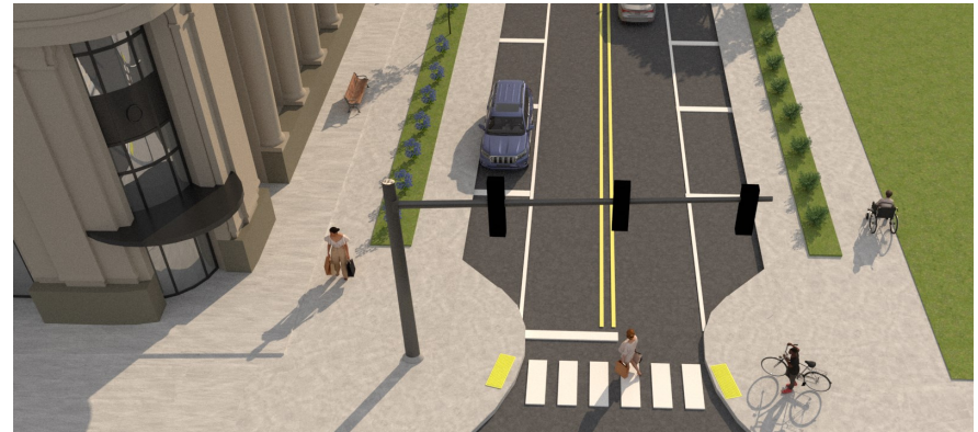
Figure 4.6.5 | Intersection with intersection nubs.
