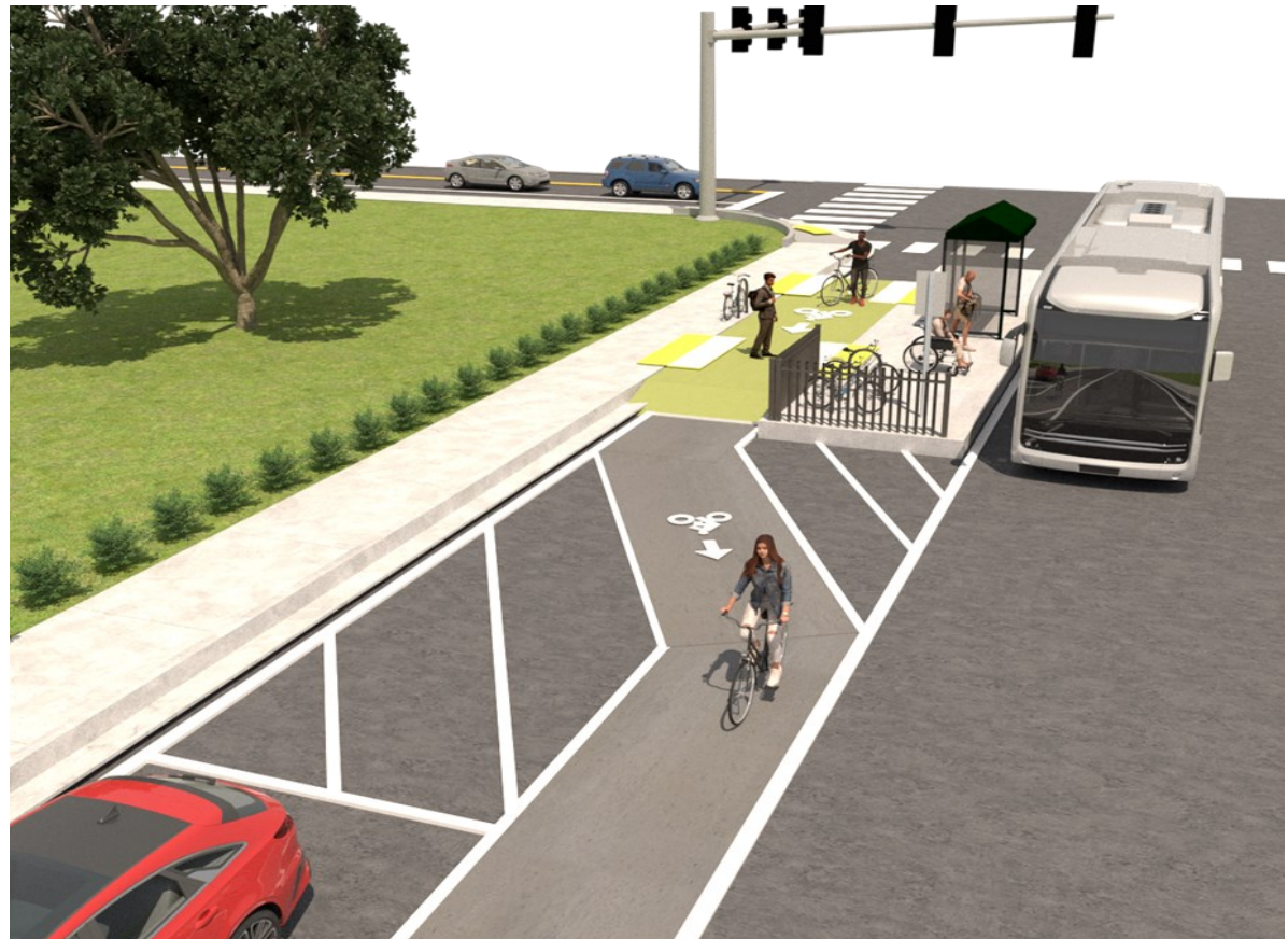
Figure 4.3.4 | Example of boarding island/floating bus stop.
