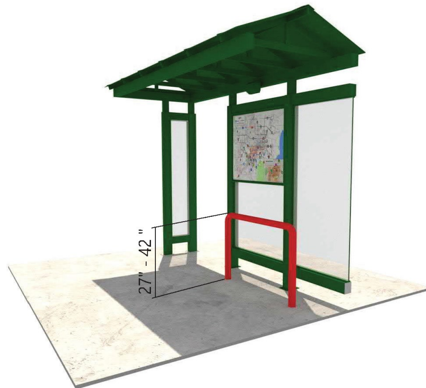
Figure 3.8.1 | Dimensions of a bus stop leaning rail.
