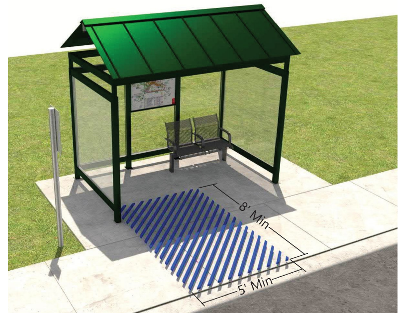
Figure 3.3.2 | Placement of bench in shelter with B&A area partially extending into shelter.
