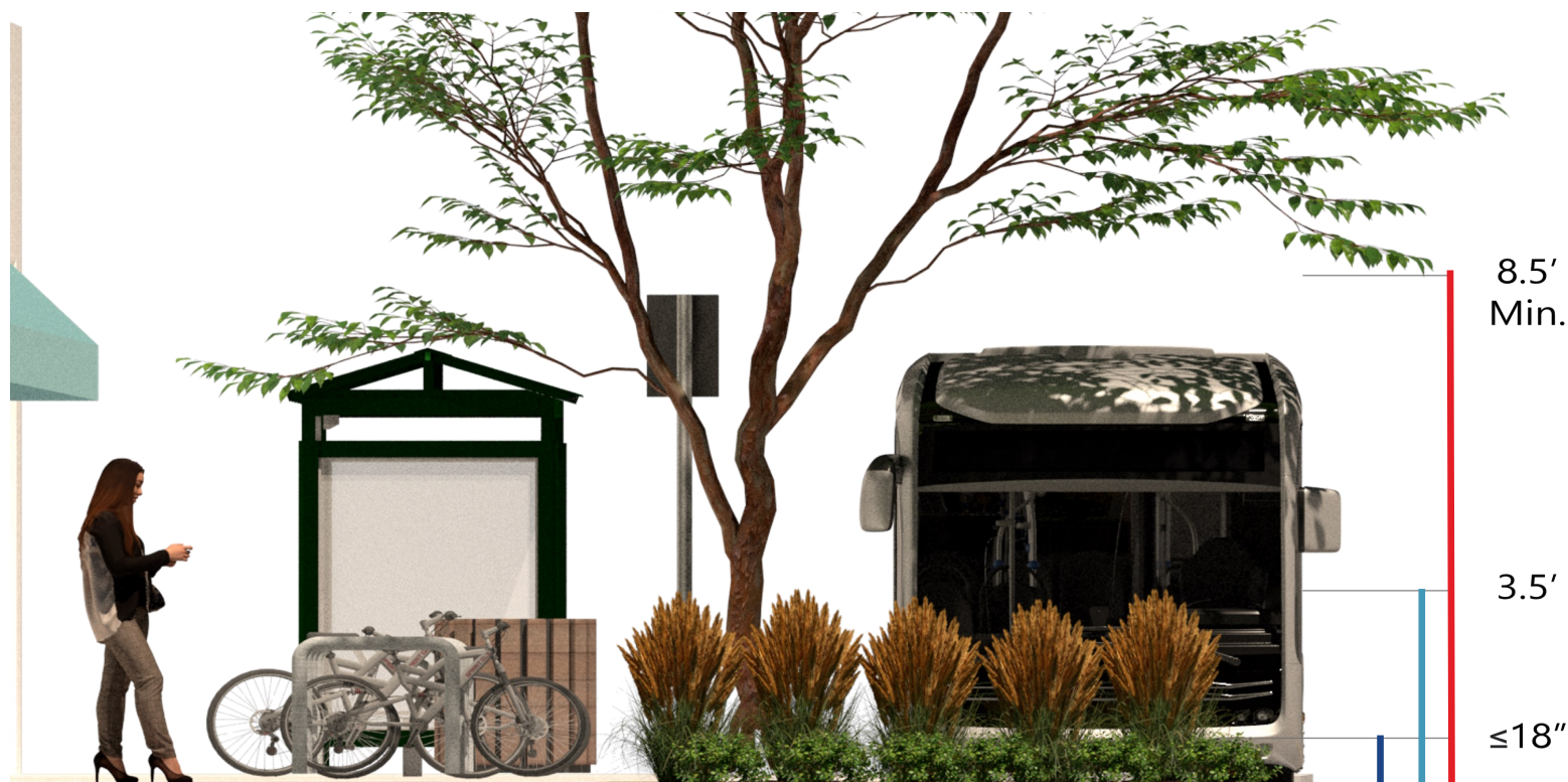
Figure 3.7.2 | Appropriate vertical dimensions for landscaping at bus stops.
