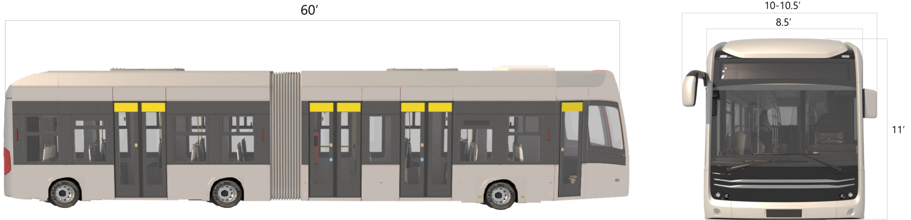
Figure 4.5.2 | Articulated bus typical dimensions.
