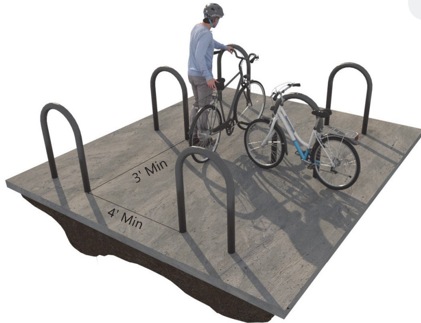
Figure 3.5.2 | Dimensions for accessible bicycle rack placement.
