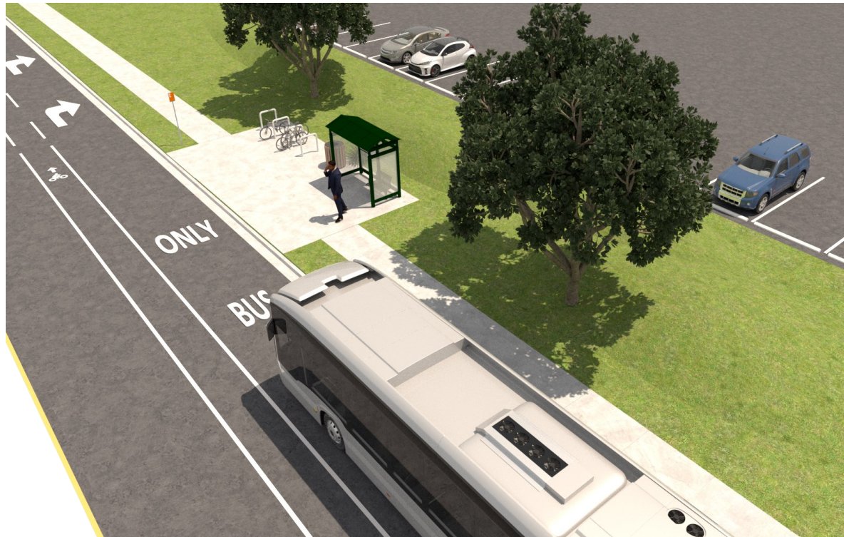
Figure 4.3.8 | Example of an open Bus Bay.
