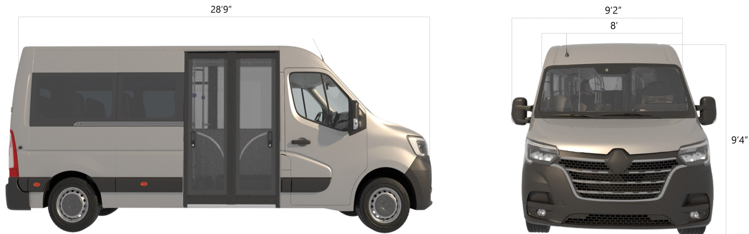
Figure 4.5.3 | On-demand or paratransit vehicle typical dimensions.
