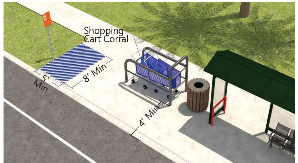
Figure 3.8.9 | Placement of a shopping cart corral at a bus stop.
