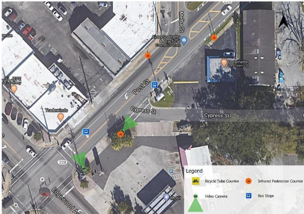
Figure 23: Device Installation Locations for Post St. North of Edgewood Ave. S (72N003)
