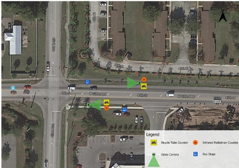
Figure 19: Device Installation Locations for N. Gifford Rd. East of 43 rd Ave. (88N003)
