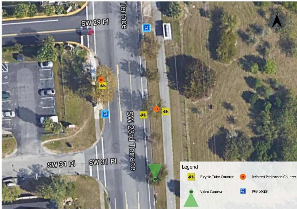
Figure 27: Device Installation Locations for Towne Park Apartments at SW 23 rd Ter. (26N007)
