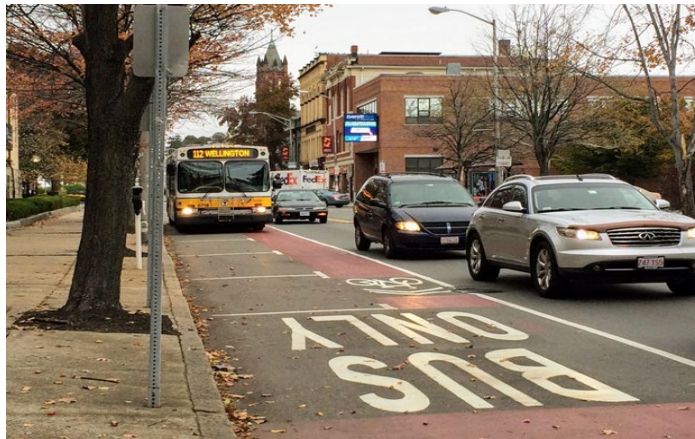
Figure 1: Example of a Pop-Up Special Use Bus Lane in Boston (Photo: UCLA ITS )
