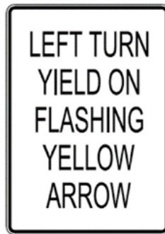
Figure 3.10-3. Flashing Yellow Arrow Sign
