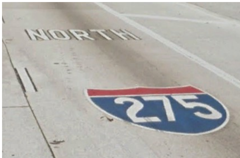
Figure 4.2-4. Cardinal Direction Markings
