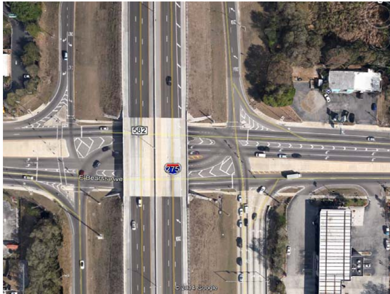
Figure 4.2-6. Dual Left Turn Lanes with Left Turn Arrows
