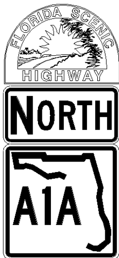
Figure 2.34-2. Co-Location on Route Confirmation Marker
