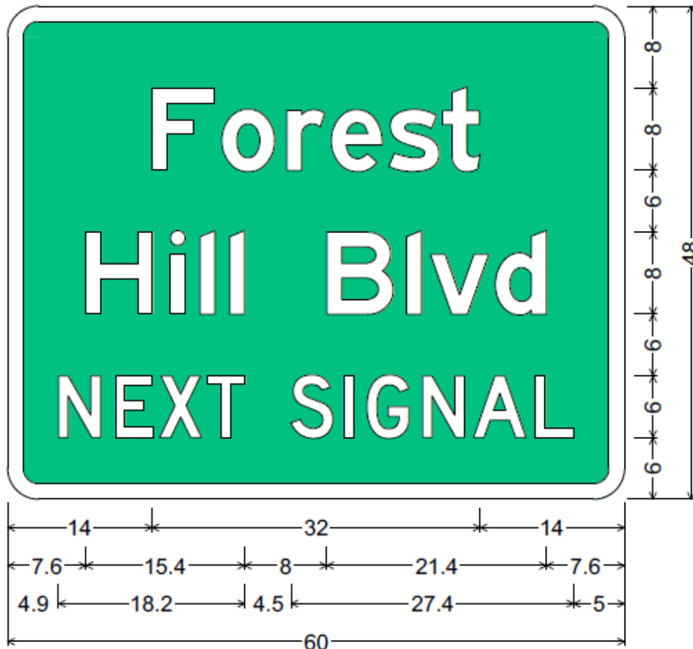
Figure 2.37-2. Advance Street Name Sign Design (Single Post)
