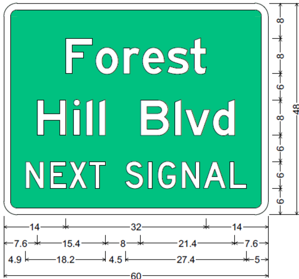
Figure 2.37-2. Advance Street Name Sign Design (Single Post)
