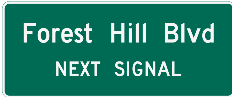
Figure 2.37-2. Advance Street Name Sign Design (Single Post)
