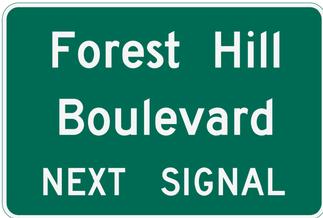
Figure 2.37-3. Advance Street Name Sign Design (Double Post)
