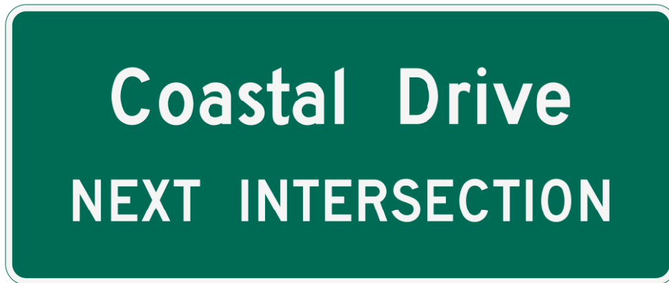
Figure 2.37-6. Advance Street Name Signs at Non-Signalized Locations
