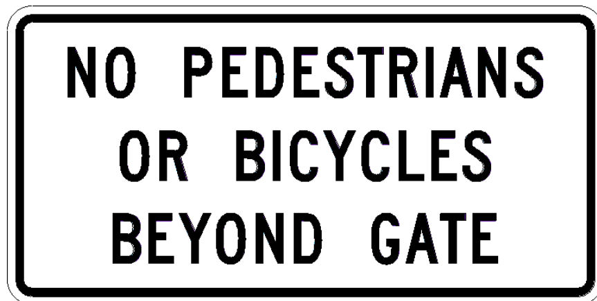
Figure 2.6-1. Swing-Style Pedestrian Gate Sign on Movable Bridges
