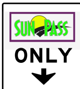
Figure 2.42-4. Priced Managed Lane Operation Sign
