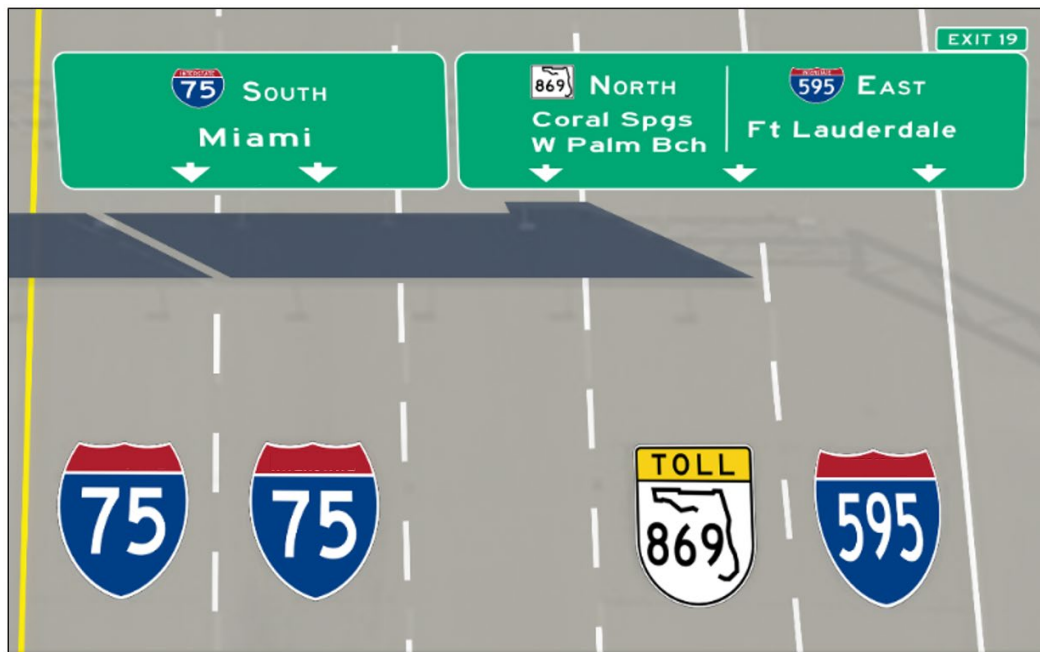
Figure 4.2-3. Route Shield Pavement Markings for Mainline
