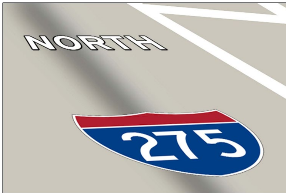
Figure 4.2-4. Cardinal Direction Markings
