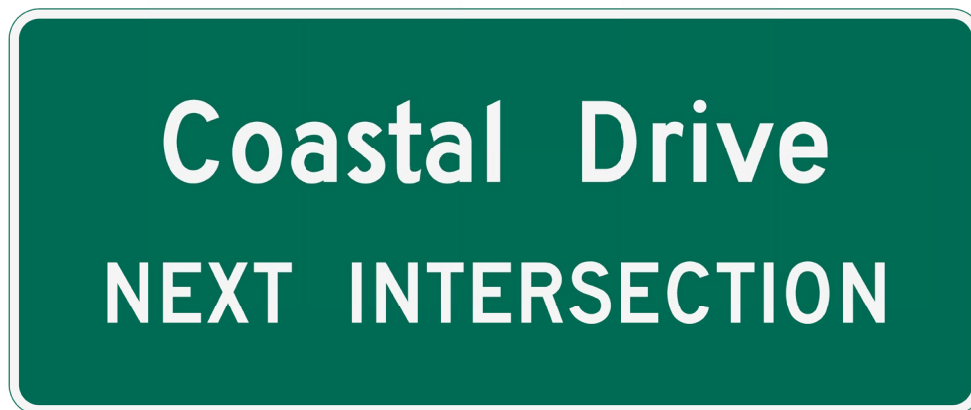
Figure 2.37-6. Advance Street Name Signs at Non-Signalized Locations
