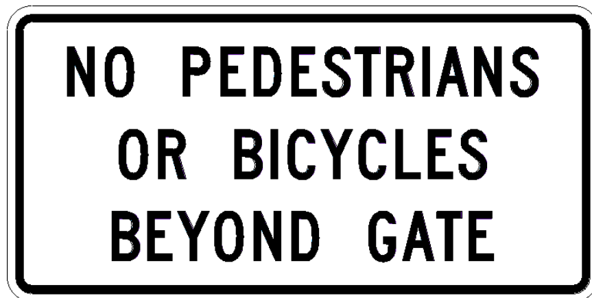
Figure 2.6-1. Swing-Style Pedestrian Gate Sign on Movable Bridges
