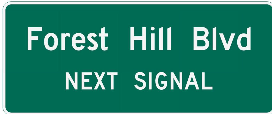
Figure 2.37-2. Advance Street Name Sign Design (Single Post)
