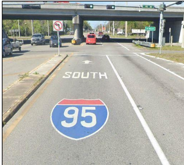
Figure 4.2-6. Pavement Markings for Interchange Access
