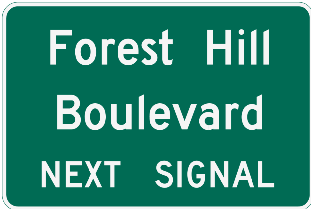
Figure 2.37-3. Advance Street Name Sign Design (Double Post)
