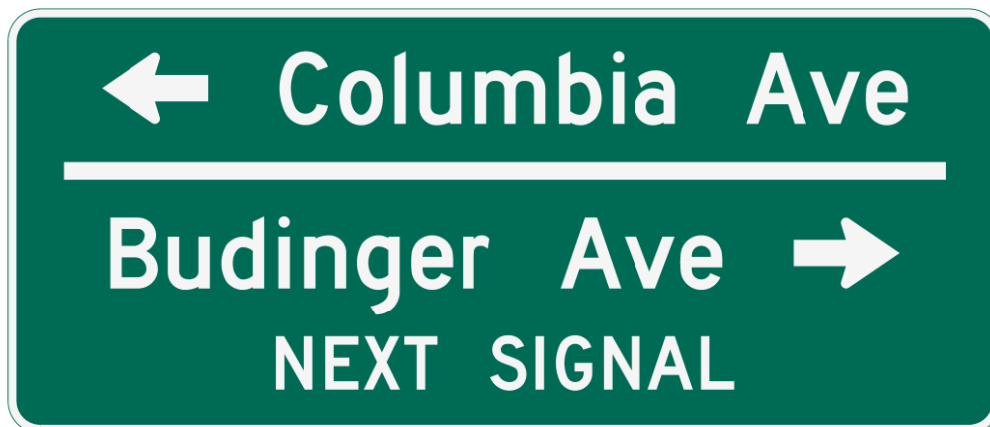
Figure 2.37-5. Advance Street Name Sign Using Different Names
