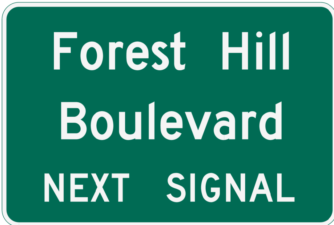
Figure 2.37-3. Advance Street Name Sign Design (Double Post)
