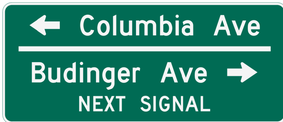
Figure 2.37-5. Advance Street Name Sign Using Different Names
