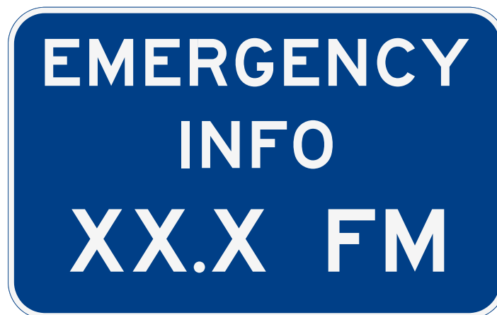
Figure 2.14-3. Radio Frequency Information Sign
