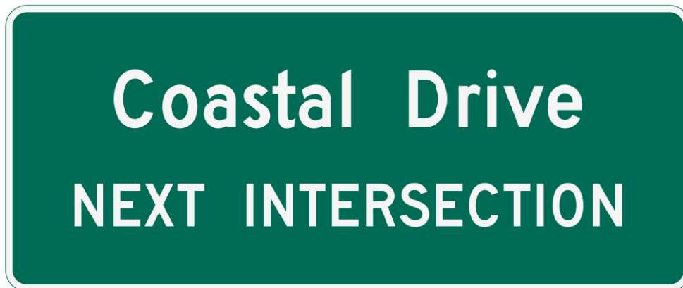
Figure 2.37-6. Advance Street Name Signs at Non-Signalized Locations
