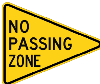
Figure 2.9-1. NO PASSING ZONE Pennant-Shaped Sign ( W14-3 )
