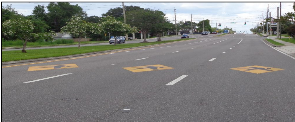
Figure 5.2-3. Pedestrian In-Pavement Warning (W11-2) Markings
