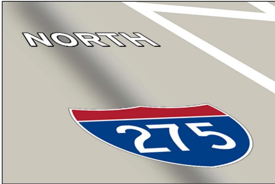
Figure 4.2-4. Cardinal Direction Markings
