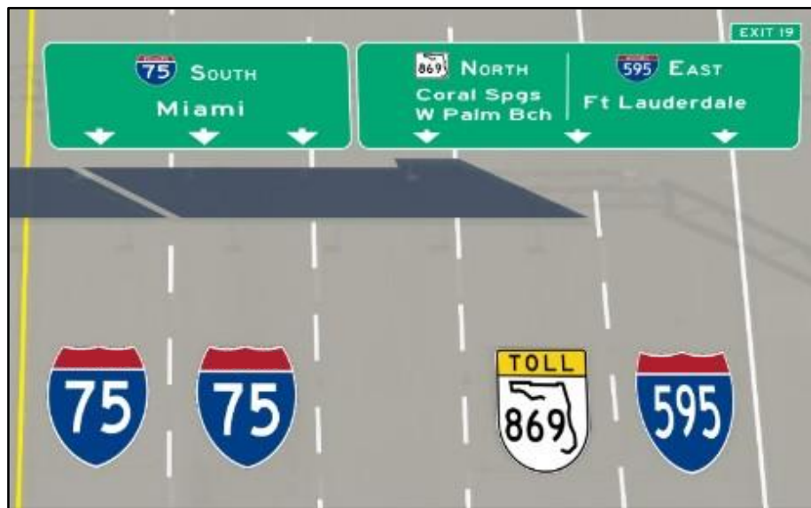
Figure 4.2-3. Route Shield Pavement Markings for Mainline
