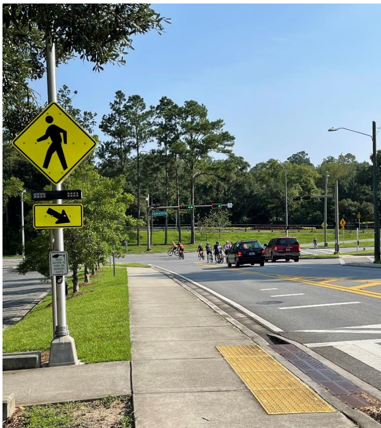
Figure 5.2-8. Rectangular Rapid Flashing Beacons (RRFB)
