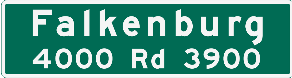
Figure 2.2-1. Overhead Street Name Sign
