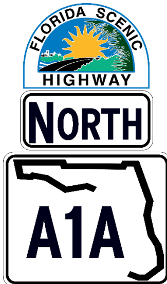
Figure 2.34-2. Co-Location on Route Confirmation Marker
