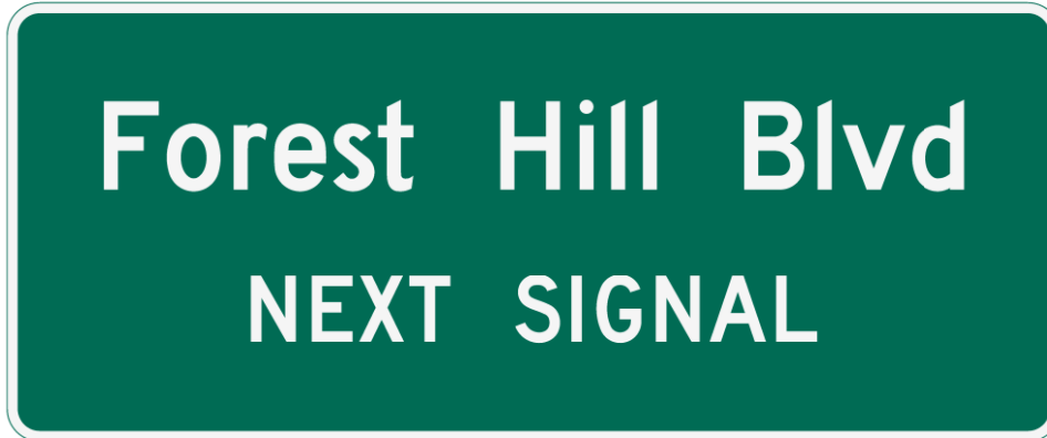
Figure 2.37-2. Advance Street Name Sign Design (Single Post)
