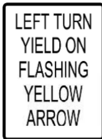
Figure 3.10-3. Flashing Yellow Arrow Sign (FTP-85-13)
