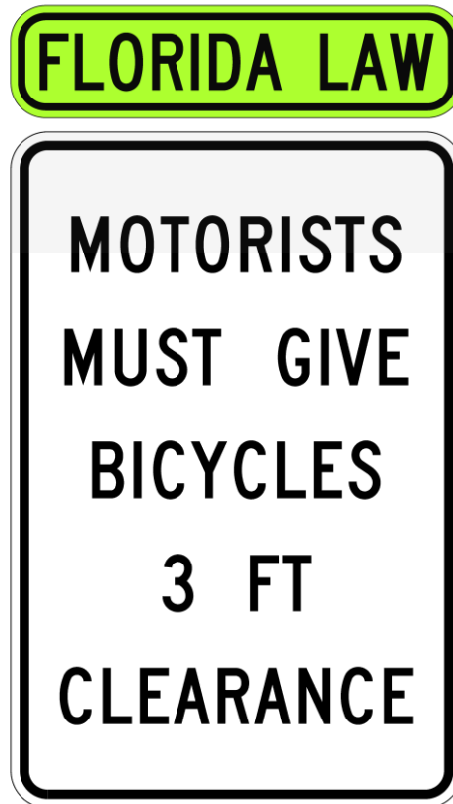
Figure 2.11-1 Bicycle Passing Clearance Sign
