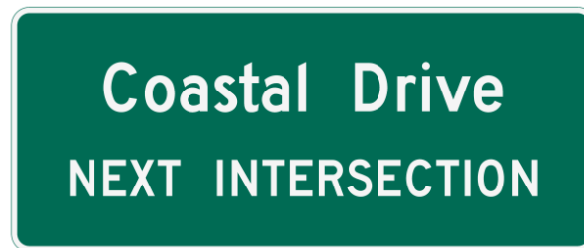
Figure 2.37-6. Advance Street Name Signs at Non-Signalized Locations
