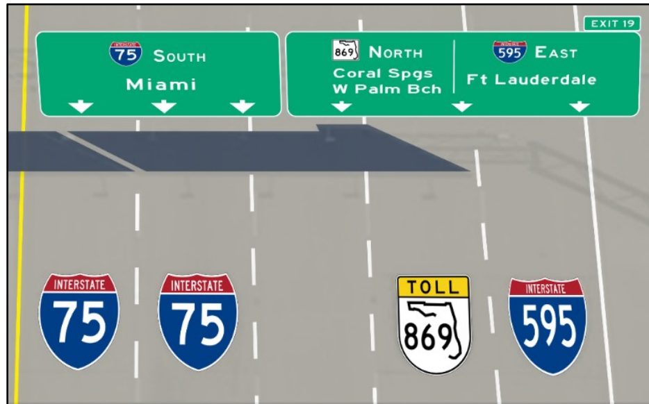
Figure 4.2-3. Route Shield Pavement Markings
