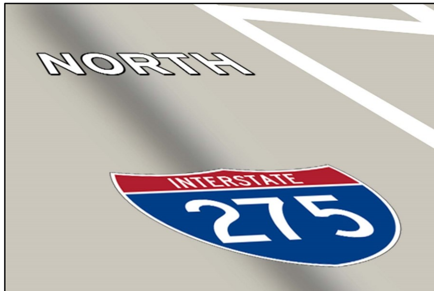
Figure 4.2-4. Cardinal Direction Markings
