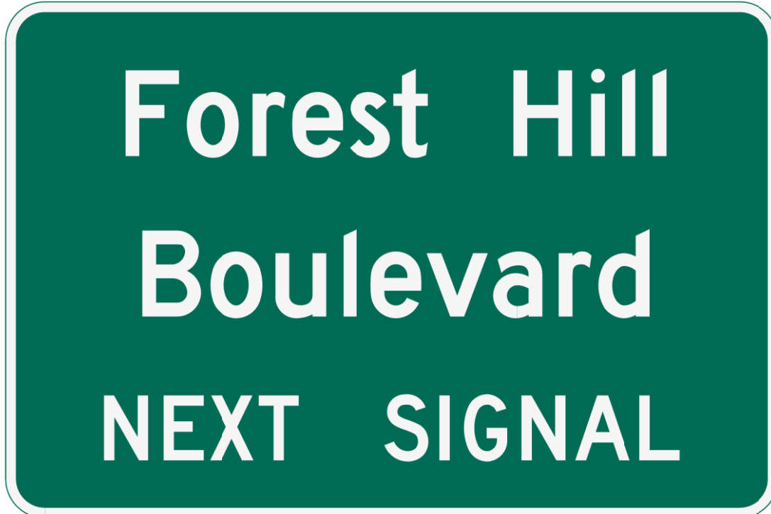
Figure 2.37-3. Advance Street Name Sign Design (Double Post)
