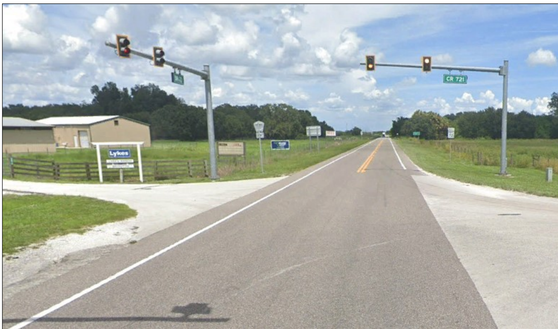
Figure 3.1-1. Intersection Control Beacon
