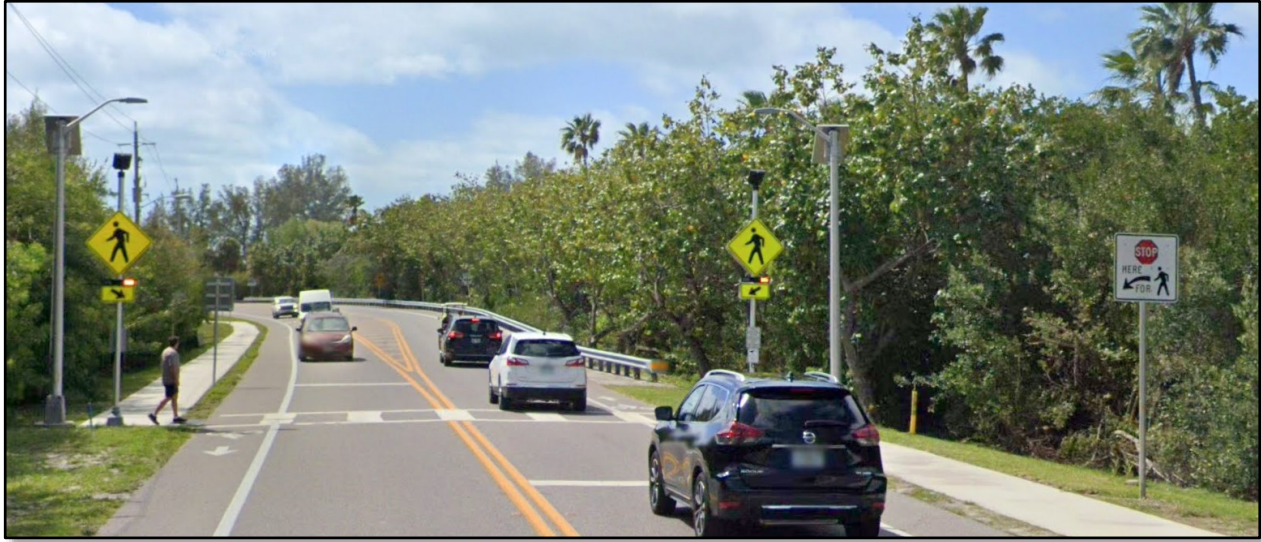
Figure 5.2-5. Pedestrian Crossing Signs (R1-5b and W11-2 with an RRFB)
