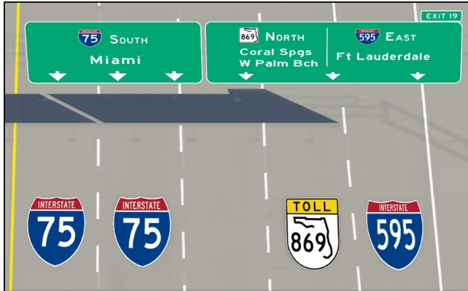
Figure 4.2-3. Route Shield Pavement Markings
