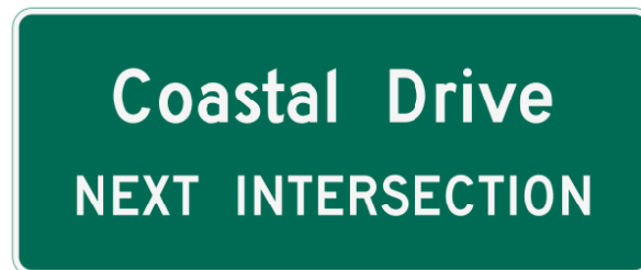
Figure 2.37-6. Advance Street Name Signs at Non-Signalized Locations
