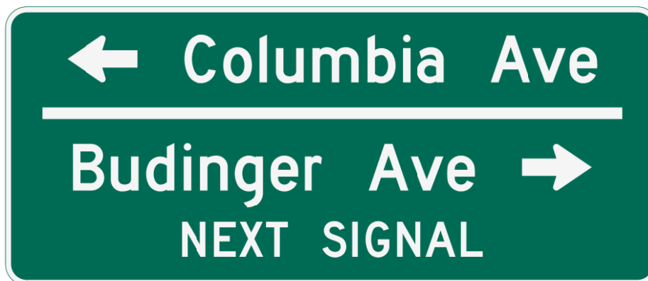
Figure 2.37-5. Advance Street Name Sign Using Different Names
