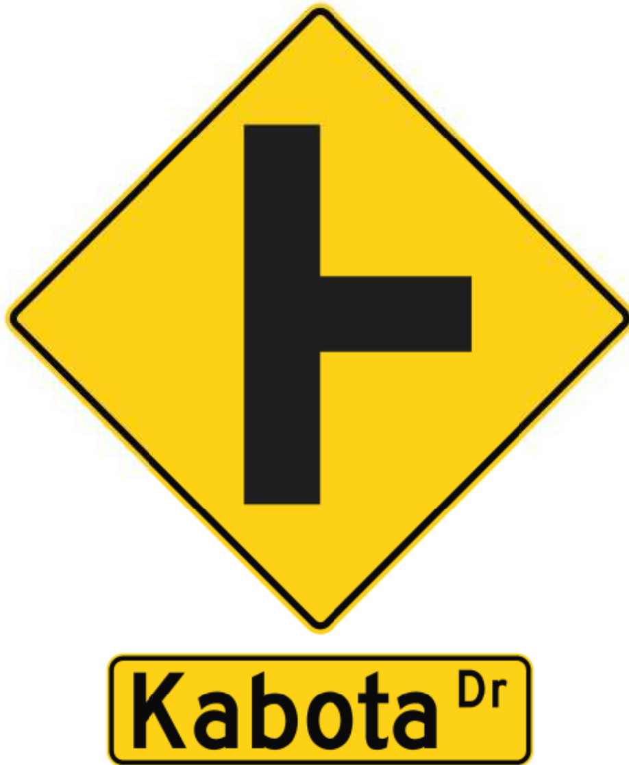
Figure 2.37-7. Advance Street Name Plaque on Intersection Warning Sign
