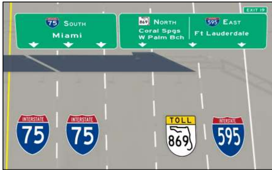
Figure 4.2-3. Route Shield Pavement Markings
