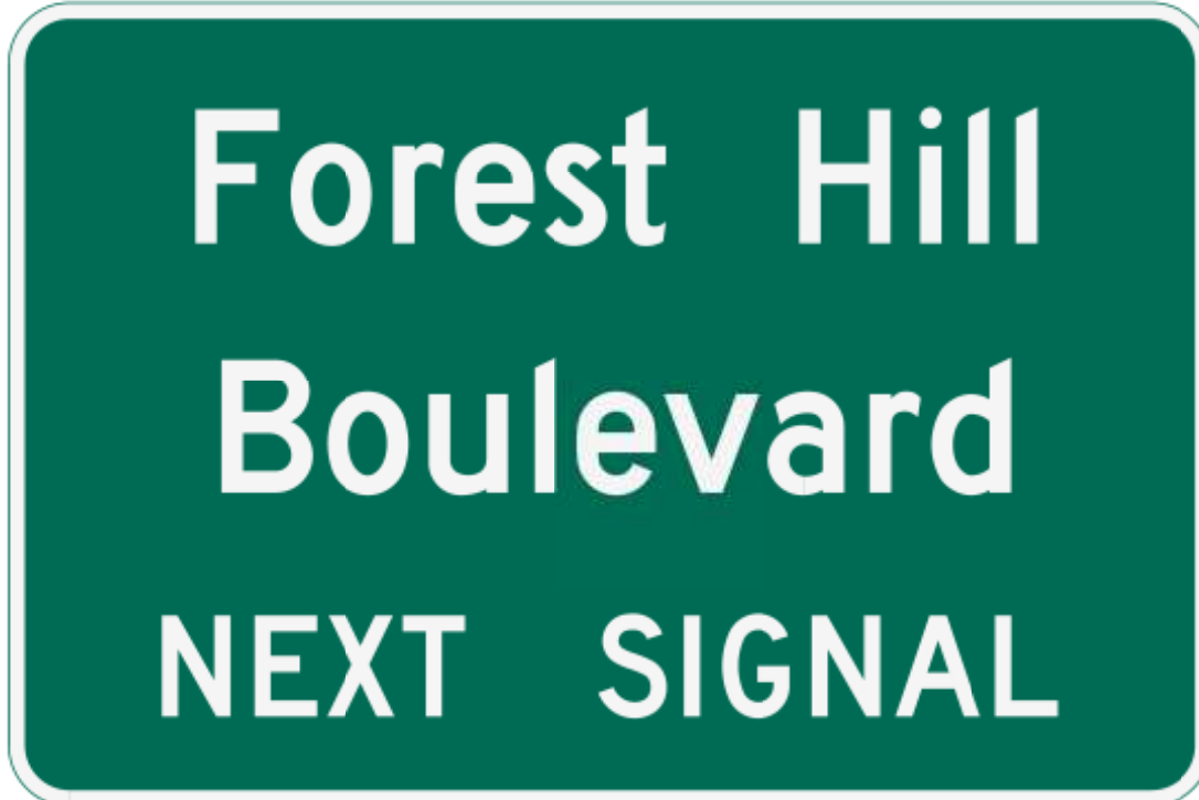
Figure 2.37-3. Advance Street Name Sign Design (Double Post)
