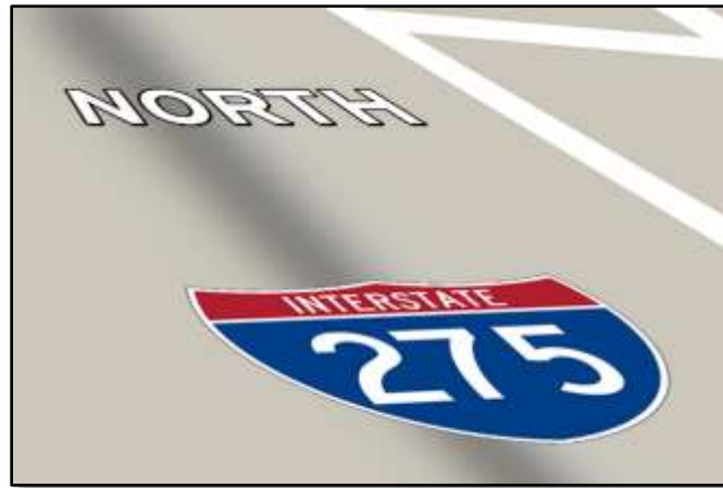
Figure 4.2-4. Cardinal Direction Markings
