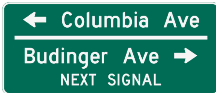
Figure 2.37-5. Advance Street Name Sign Using Different Names
