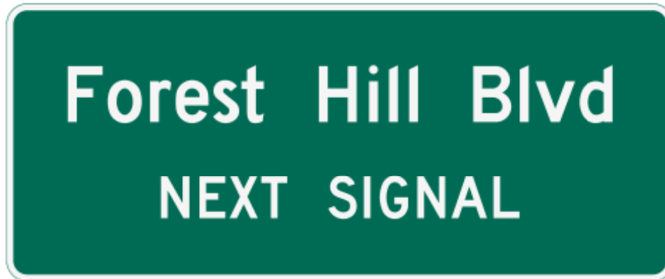
Figure 2.37-2. Advance Street Name Sign Design (Single Post)
