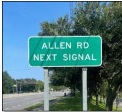
Figure 2.37-1. Advance Street Name Sign at Signalized Locations
