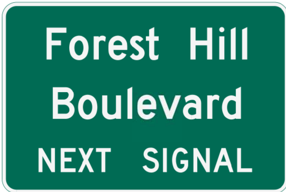
Figure 2.37-3. Advance Street Name Sign Design (Double Post)
