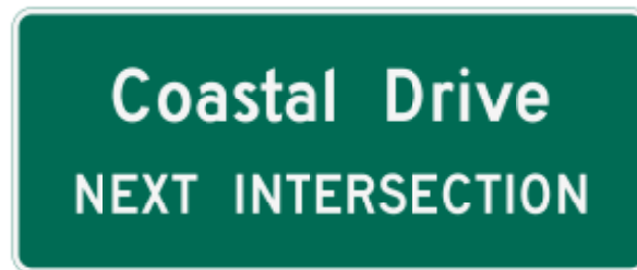
Figure 2.37-6. Advance Street Name Signs at Non-Signalized Locations
