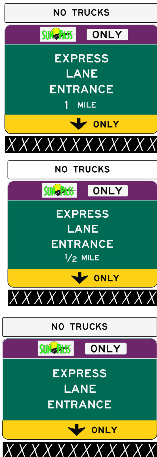
Figure 2.42-5. Examples of Ingress Signing
