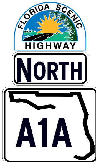
Figure 2.34-2. Co-Location on Route Confirmation Marker
