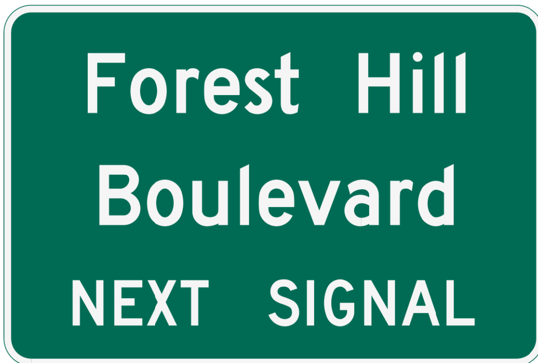
Figure 2.37-3. Advance Street Name Sign Design (Double Post)
