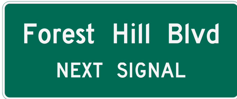
Figure 2.37-2. Advance Street Name Sign Design (Single Post)
