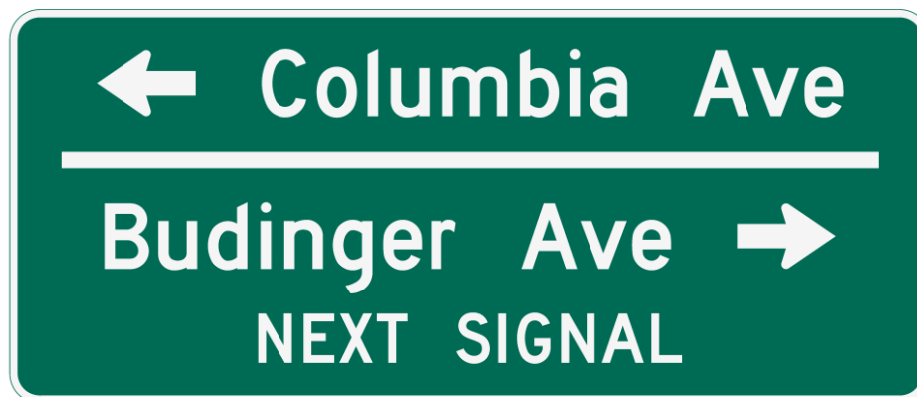
Figure 2.37-5. Advance Street Name Sign Using Different Names
