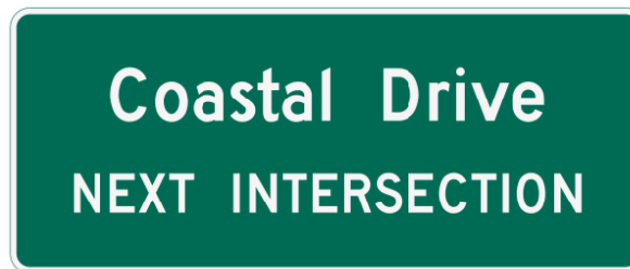
Figure 2.37-6. Advance Street Name Signs at Non-Signalized Locations
