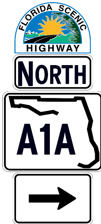
Figure 2.34-3. Co-Location on Route Direction Marker
