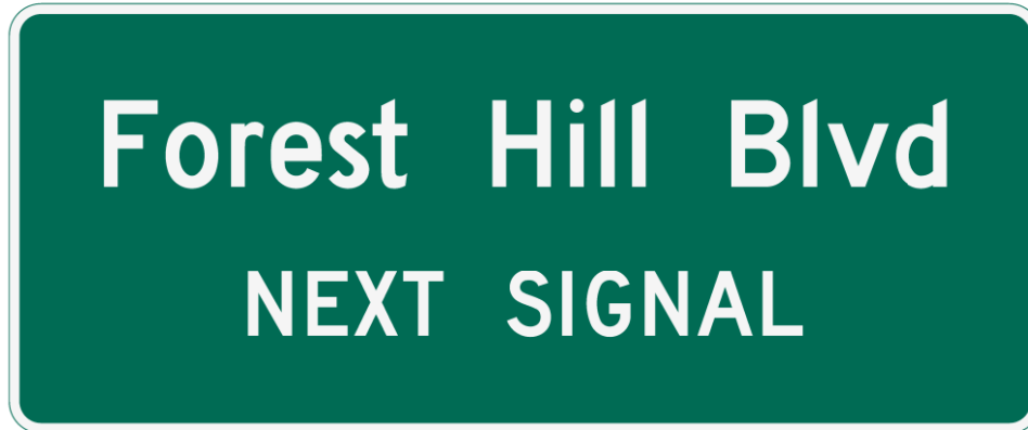
Figure 2.37-2. Advance Street Name Sign Design (Single Post)
