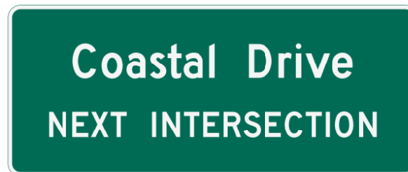
Figure 2.37-6. Advance Street Name Signs at Non-Signalized Locations
