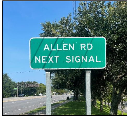
Figure 2.37-1. Advance Street Name Sign at Signalized Locations
