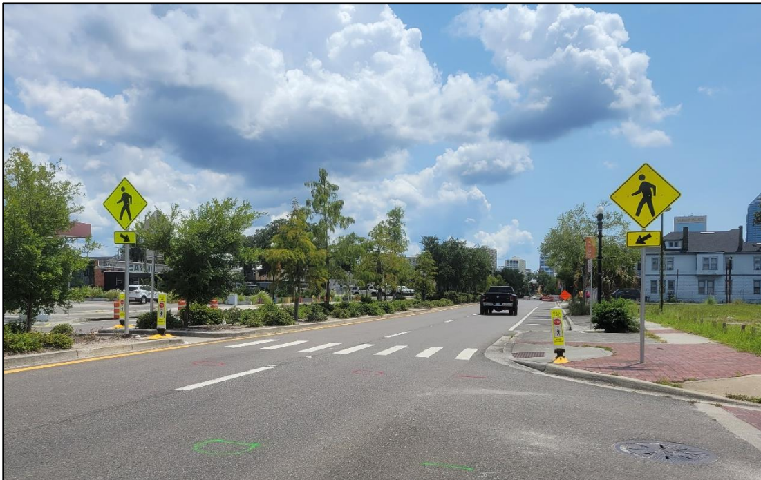
Figure 5.2-6. Pedestrian Crossing Signs (R1-6a and W11-2)
