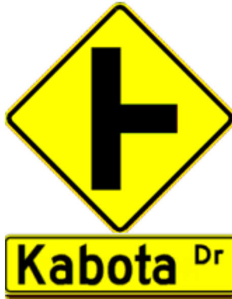
Figure 2.37-7. Advance Street Name Plaque on Intersection Warning Sign
