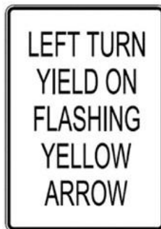
Figure 3.10-3. Flashing Yellow Arrow Sign
