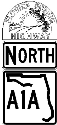
Figure 2.34-2. Co-Location on Route Confirmation Marker
