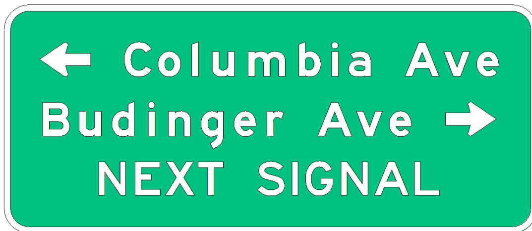
Figure 2.37-5. Advance Street Name Sign Using Different Names
