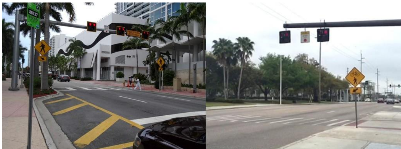
Figure 3.8-3. Pedestrian Hybrid Beacons
