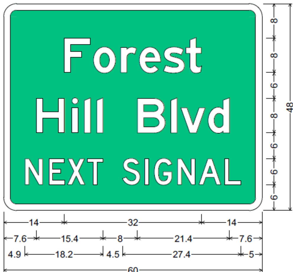
Figure 2.37-2. Advance Street Name Sign Design (Single Post)
