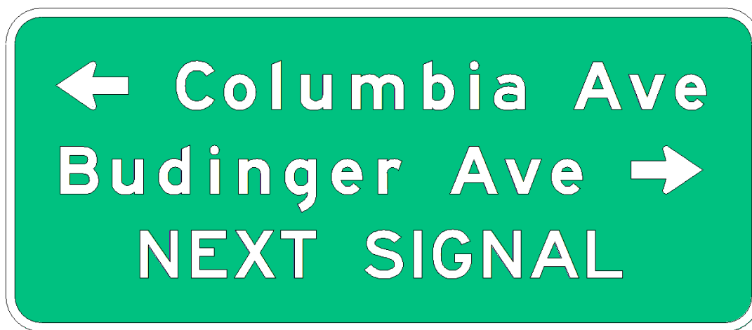
Figure 2.37-5. Advance Street Name Sign Using Different Names
