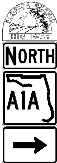
Figure 2.34-3. Co-Location on Route Direction Marker
