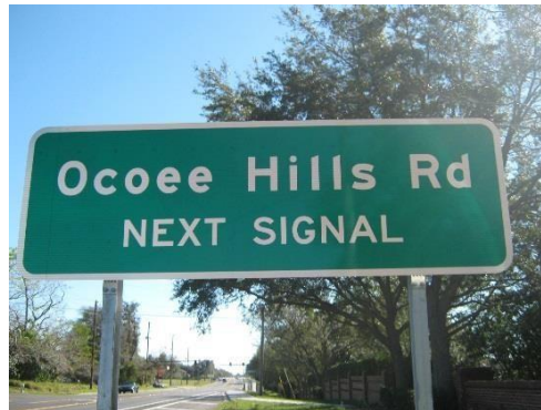
Figure 2.37-1. Advance Street Name Sign at Signalized Locations
