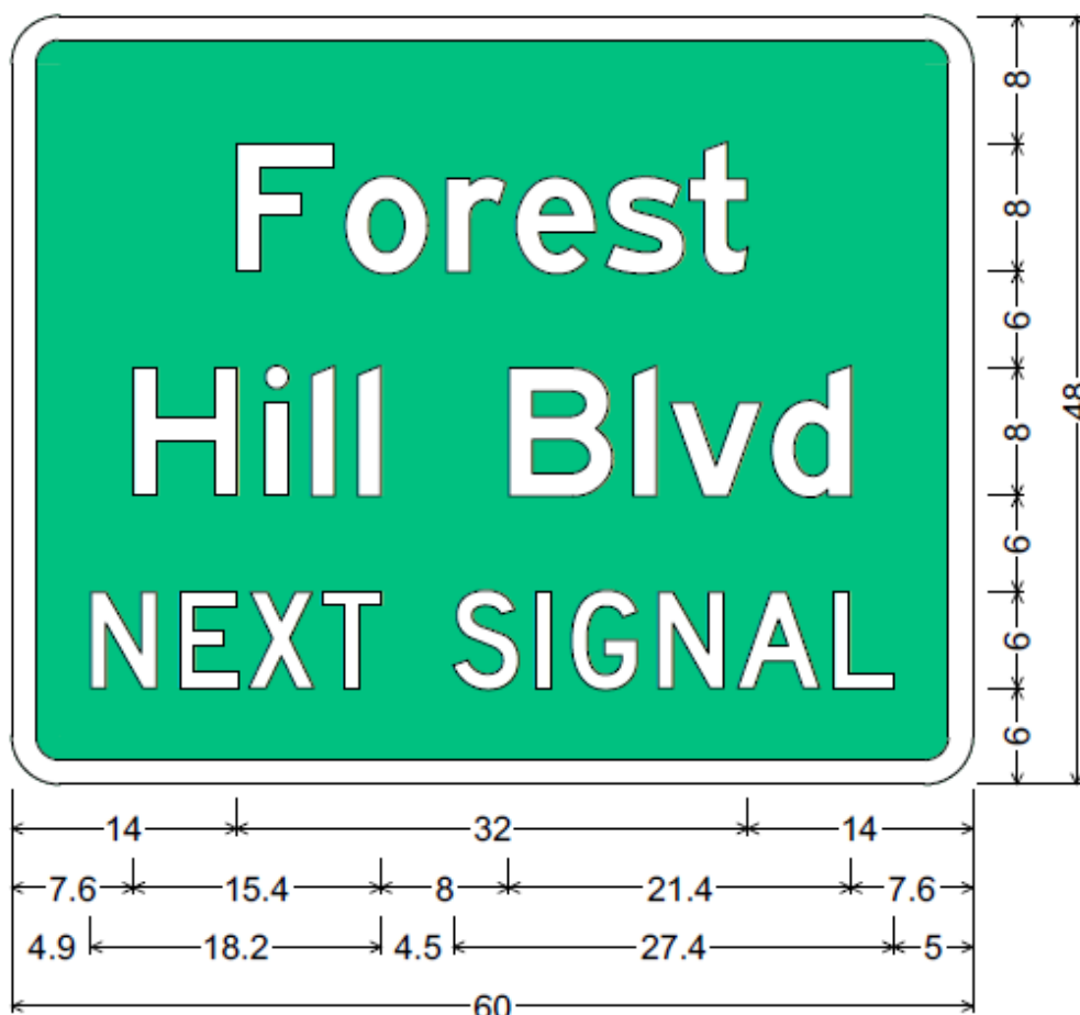
Figure 2.37-2. Advance Street Name Sign Design (Single Post)
