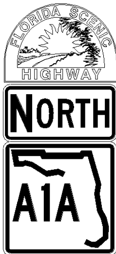
Figure 2.34-2. Co-Location on Route Confirmation Marker
