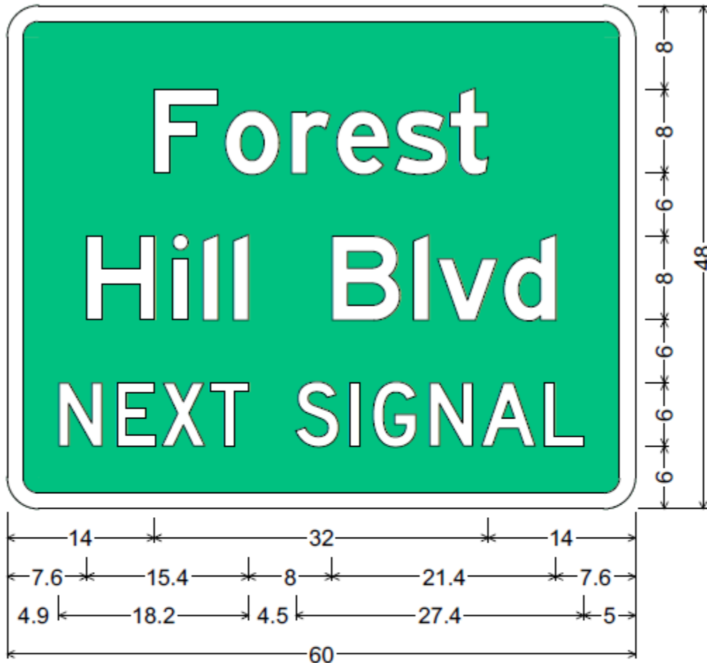
Figure 2.37-3. Advance Street Name Sign Design (Single Post)
