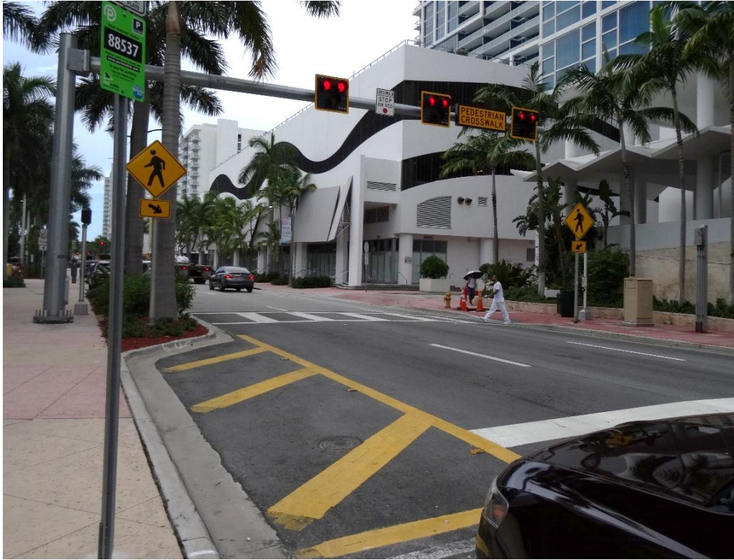
Figure 3.8.2. Pedestrian Hybrid Beacons
