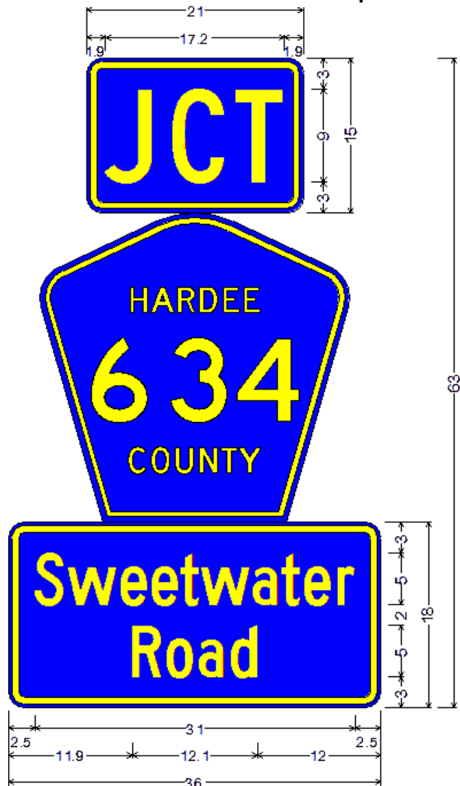
Figure 2.37-10. Advance Street Name Plaque on Advanced Route Marker
