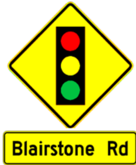
Figure 2.37-9. Advance Street Name Plaque on Advance Traffic Control Warning Sign
