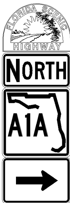
Figure 2.34-3. Co-Location on Route Direction Marker
