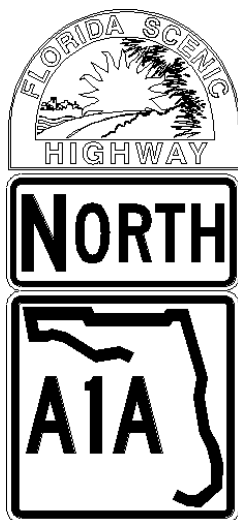
Figure 2.34-2. Co-Location on Route Confirmation Marker
