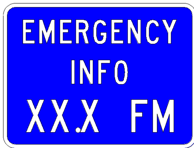
Figure 2.14-5. Radio Frequency Information Sign
