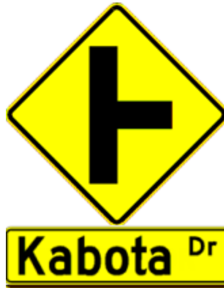
Figure 2.37-8. Advance Street Name Plaque on Intersection Warning Sign
