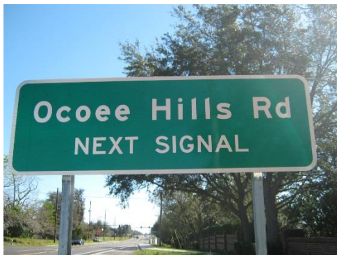
Figure 2.37-1. Advance Street Name Sign at Signalized Locations
