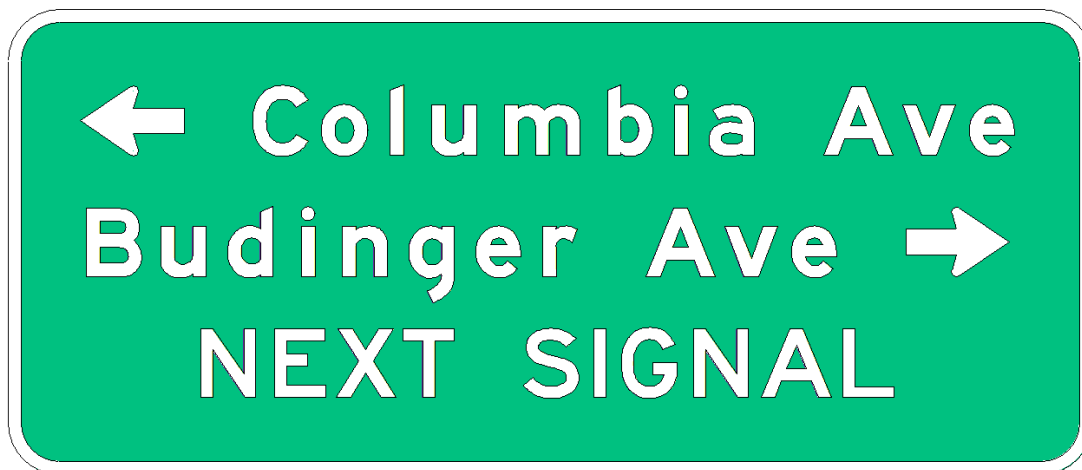
Figure 2.37-6. Advance Street Name Sign Using Different Names
