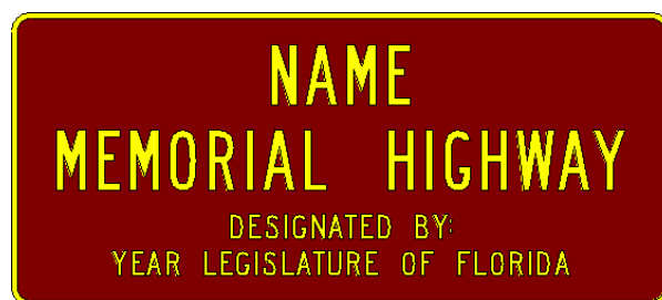
Figure 2.35-1. Memorial Roadway Designation Sign
