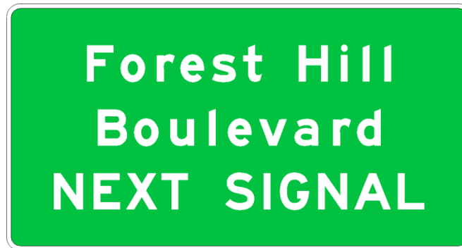
Figure 2.37-1. Advance Street Name Sign at Signalized Locations
