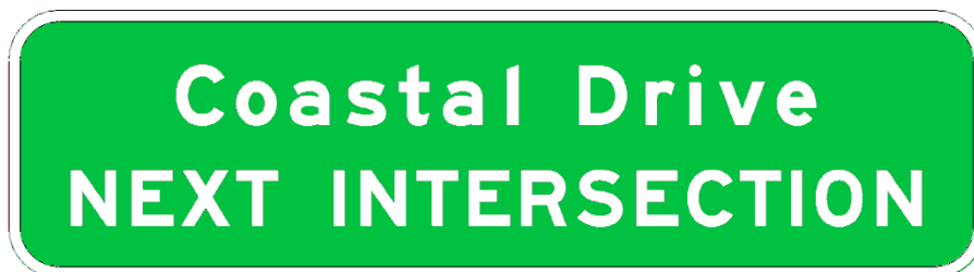
Figure 2.37-4. Advance Street Name Signs at Non-Signalized Locations
