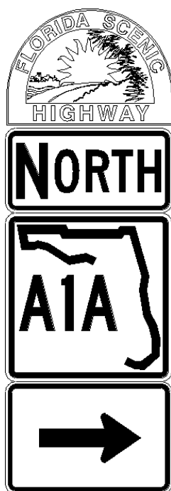
Figure 2.34-3. Co-Location on Route Direction Marker
