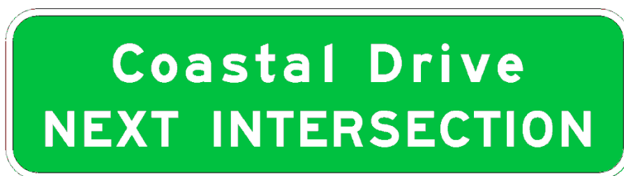
Figure 2.37-4. Advance Street Name Signs at Non-Signalized Locations
