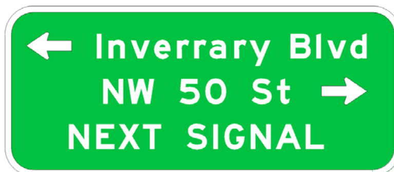
Figure 2.37-3. Advance Street Name Sign Using Different Names
