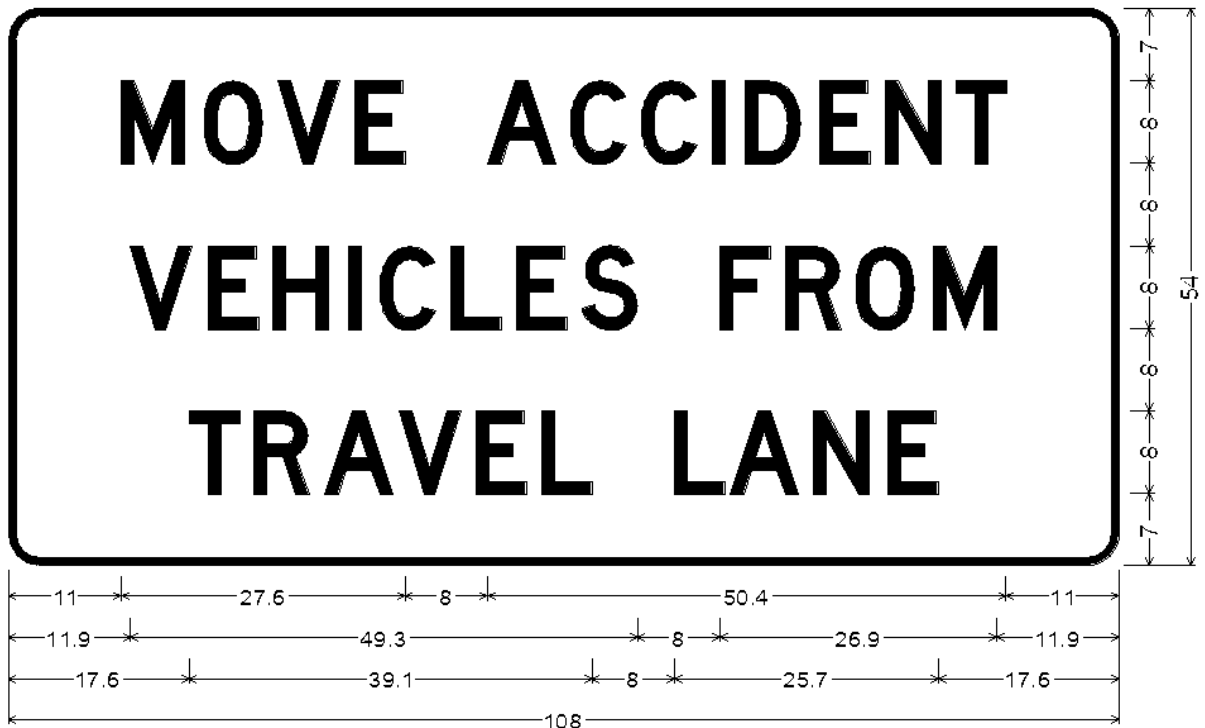
Figure 2.8-1. FTP-28-04; 3.0" Radius, 0.8" Border, Black on White; "MOVE ACCIDENT" D; "VEHICLES FROM" D; "TRAVEL LANE" D;
