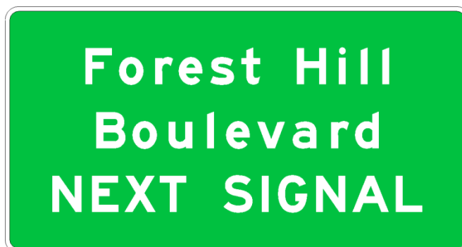
Figure 2.37-1. Advance Street Name Sign at Signalized Locations
