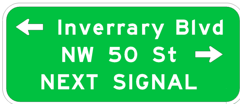
Figure 2.37-3. Advance Street Name Sign Using Different Names
