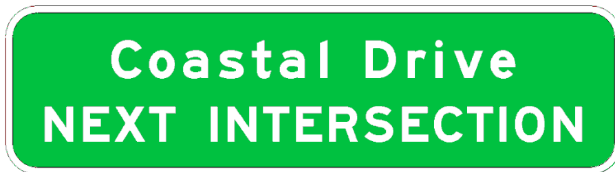
Figure 2.37-4. Advance Street Name Signs at Non-Signalized Locations
