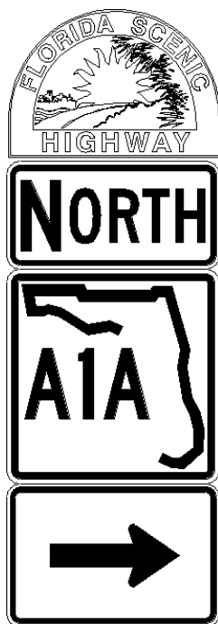
Figure 2.34-3. Co-Location on Route Direction Marker
