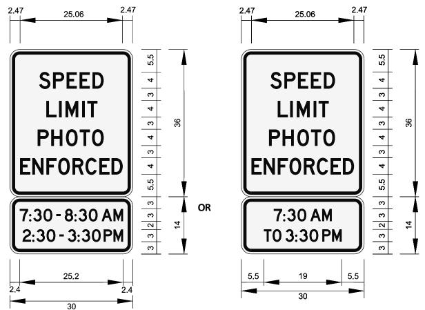
FTP - MINIMUM, SPEED LIMIT PHOTO ENFORCED; 1.875" Radius, 0.787" Border, 0.475" Indent, Black on White; "SPEED" D 2K; "LIMIT" D 2K;
