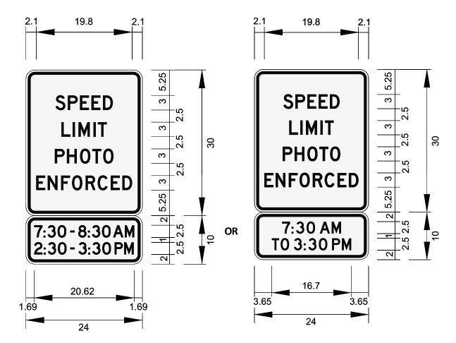
FTP - MINIMUM, SPEED LIMIT PHOTO ENFORCED; 1.5" Radius, 0.63" Border, 0.38" Indent, Black on White; "SPEED" D 2K;
