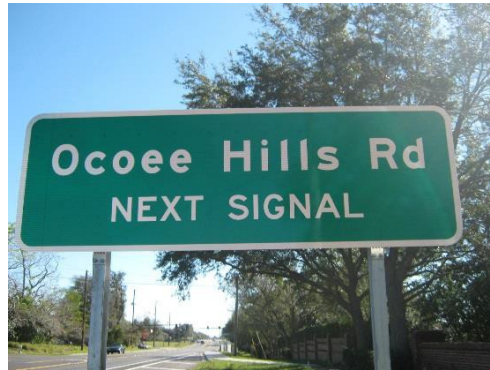
Figure 2.37-1. Advance Street Name Sign at Signalized Locations
