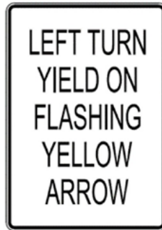
Figure 3.10-3. Flashing Yellow Arrow Sign
