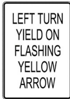
Figure 3.10-3. Flashing Yellow Arrow Sign
