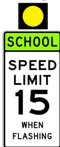
Figure 15-7A 15 MPH School Zone Roadside Flashing Beacon Assembly (MUTCD S5-1)
