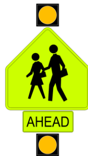
Figure 15-11 School Advance Crossing Sign with Flashing Beacon Assembly Used for Additional School Zone Warning on Multilane Roadways
