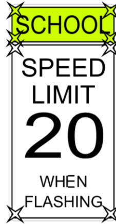
Figure 15-8B 20 MPH Highlighted School Zone Roadside Sign Assembly with Flashing Light Emitting Diodes (LEDs)
