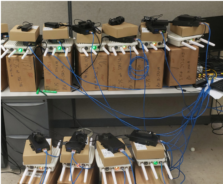
RSUs being provisioned with MAP, other applications, and credentials for the SCMS.
