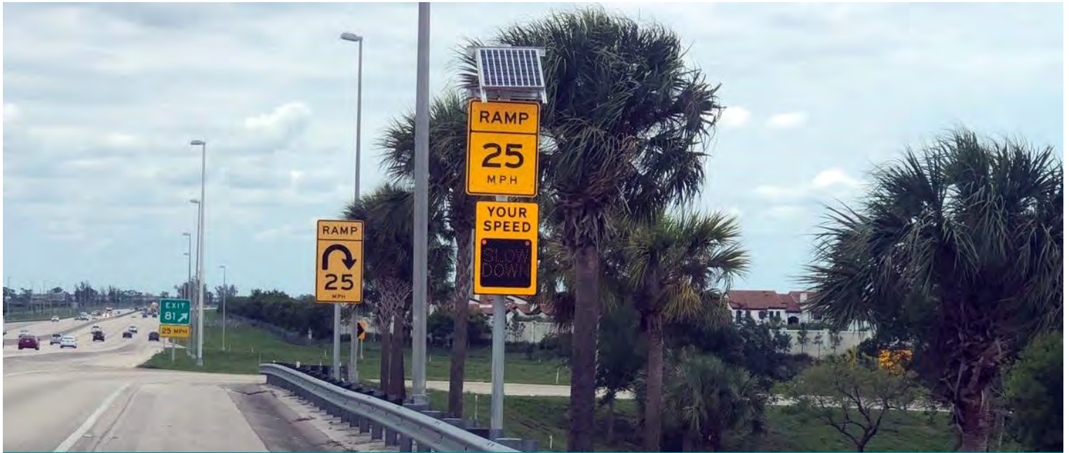
Highlighted Speed Feedback Sign on the Atlantic Avenue Exit Ramp, Turnpike Mainline Exit 81
