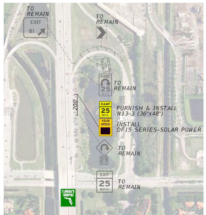
Sample Plan Sheet Used During Installation of Feedback Signage at Atlantic Avenue.
