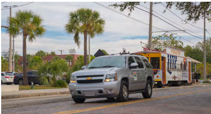
A vehicle with Connected Vehicle technology installed prepares to turn in front of a TECO streetcar to demonstrate the streetcar conflict technology. Drivers in both the vehicle and the streetcar will hear and see an alert warning them of a possible collision.
