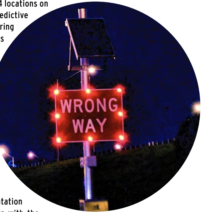
LED "Wrong Way Driver Detection" master unit during night time testing
