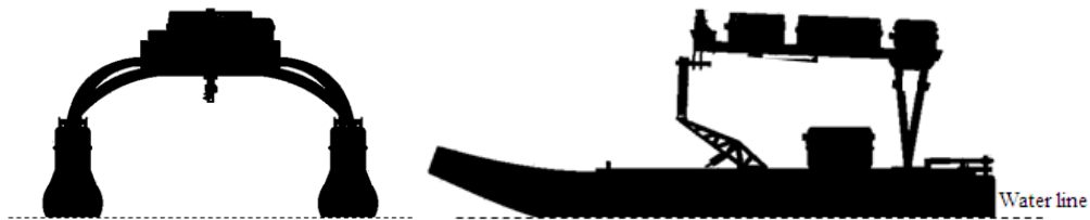
Figure 28: Frontal (left) and lateral (right) projected areas.
