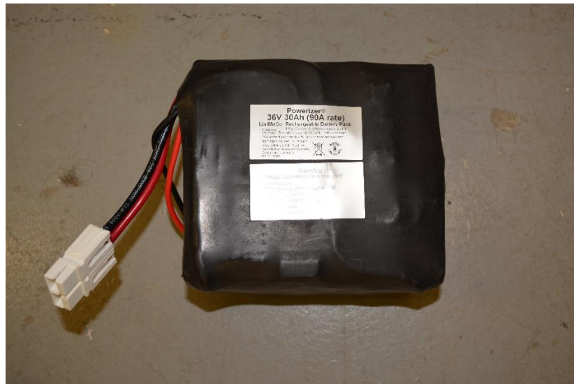
Figure 12: The LiNiMnCo 36 V, 30 Ah batteries.
