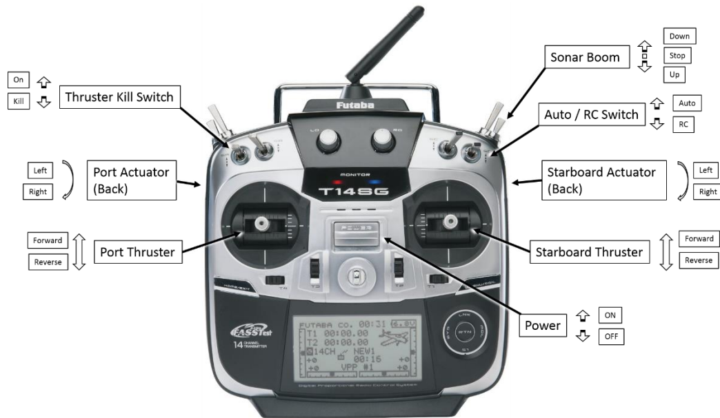
Figure 50: Configuration of the hand-held RC Control unit.
