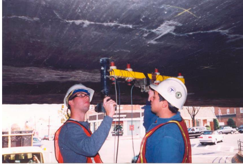
Figure 3: Acoustic sensing system [31].
