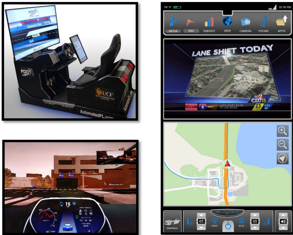
Figure 5 : Version 2.0 of the FDOT-CAVS. Top Left: A side view of the complete simulator system. Right: The complete interactive dashboard console display showing the routing and media player panes. Bottom-left: A view from the main screen of the simulator as the car approaches a parking garage. The dashboard iconography replicates (with permission) that of the Tesla Model S.
