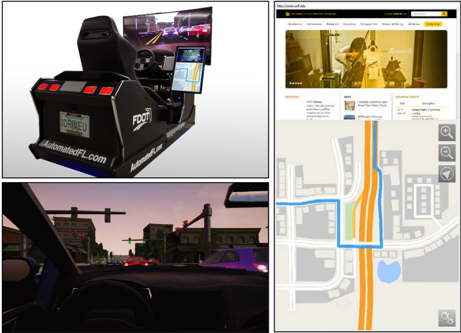
Figure 2 : Version 1.0 of the FDOT-CAVS. This testbed is an advanced simulator used for measuring human experiences with connected vehicles. Top Left: A side view of the complete simulator system demonstrated on October 10, 2015. Right: The complete interactive dashboard console display showing the web-browser and navigation panes. Bottom-left: A view from the main screen of the simulator as the car approaches an intersection.
