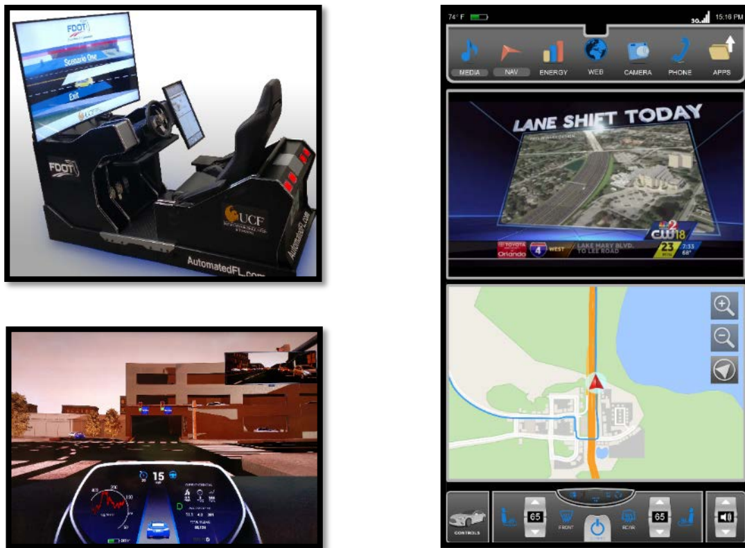
Figure 13: The FDOT DCVS is an advanced simulator used for measuring human experiences with connected vehicles. Top Left: A side view of the complete simulator system. Right: The complete interactive dashboard console display showing the routing and media player panes. Bottom-left: A view from the main screen of the simulator as the car approaches a parking garage. The dashboard iconography replicates (with permission) that of the Tesla Model S.
