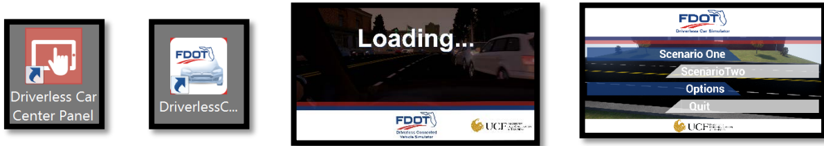
Figure 22: Launching the Application. From Left. First: The Center Panel icon launches the navigation and entertainment interface. Second: The DriverlessCar Icon launches the DCVS. Third: The Loading screen for the simulator. Fourth: The main menu of the simulator offers three options: Play Scenario 1, Play Scenario 2, or Exit the program.
