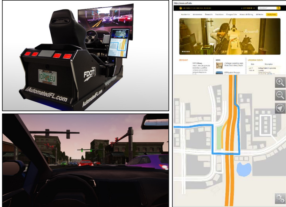
Figure 8: The FDOT DCVS is an advanced simulator used for measuring human experiences with connected vehicles. Top Left: A side view of the complete simulator system demonstrated on October 10, 2015. Right: The complete interactive dashboard console display showing the web-browser and navigation panes. Bottom-left: A view from the main screen of the simulator as the car approaches an intersection.
