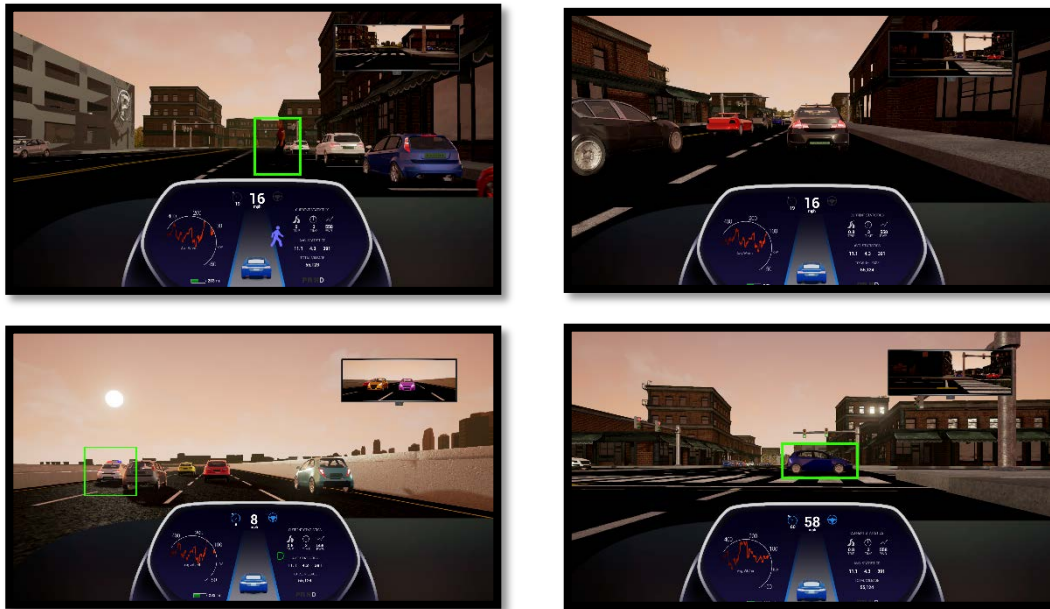
Figure 6 : Hazardous Road Conditions. Top Left: The driverless car stops as a pedestrian walks across the street. Top Right: The driverless car navigates heavy traffic in the busy downtown. Bottom Left: Traffic on the highway abruptly slows to a crawl as the police car activates its sirens. Bottom Right: The driverless car brakes abruptly as another car runs a red light.
