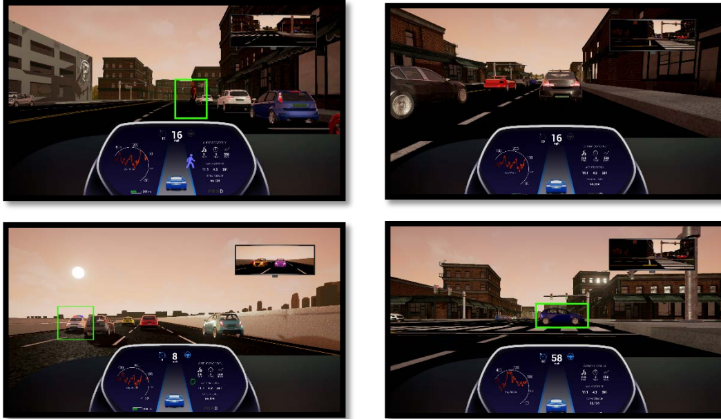
Figure 20: Hazardous Road Conditions. Top Left: The driverless car stops as a pedestrian walks across the street. Top Right: The driverless car navigates heavy traffic in the busy downtown. Bottom Left: Traffic on the highway abruptly slows to a crawl as the police car activates its sirens. Bottom Right: The driverless car brakes abruptly as another car runs a red light.
