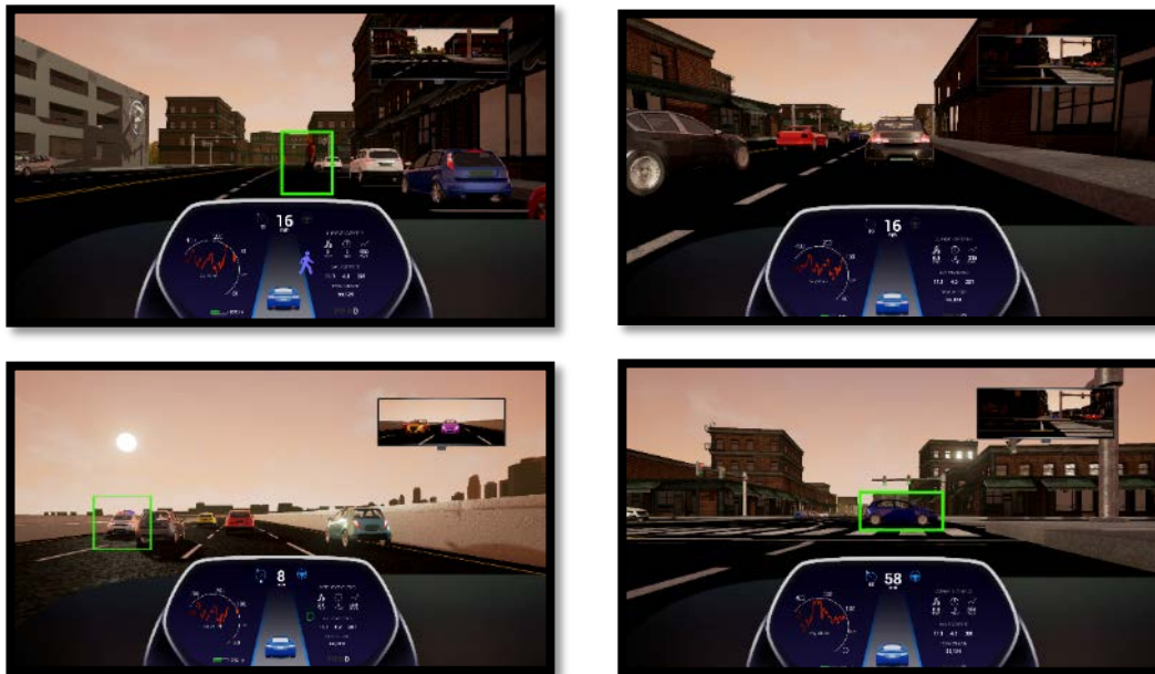
Figure 14: Hazardous Road Conditions. Top Left: The driverless car stops as a pedestrian walks across the street. Top Right: The driverless car navigates heavy traffic in the busy downtown. Bottom Left: Traffic on the highway abruptly slows to a crawl as the police car activates its sirens. Bottom Right: The driverless car brakes abruptly as another car runs a red light.
