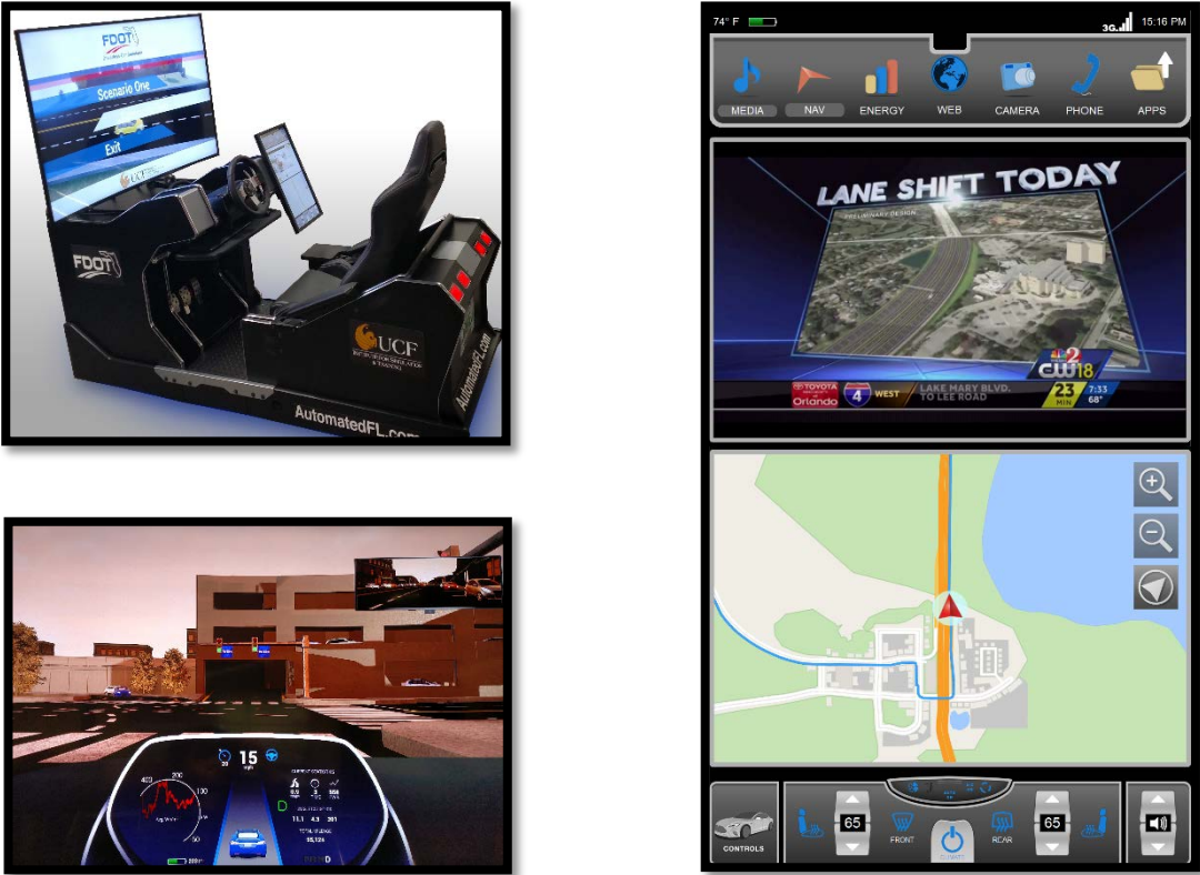
Figure 19: The FDOT DCVS is an advanced simulator used for measuring human experiences with connected vehicles. Top Left: A side view of the complete simulator system. Right: The complete interactive dashboard console display showing the routing and media player panes. Bottom-left: A view from the main screen of the simulator as the car approaches a parking garage. The dashboard iconography replicates (with permission) that of the Tesla Model S.
