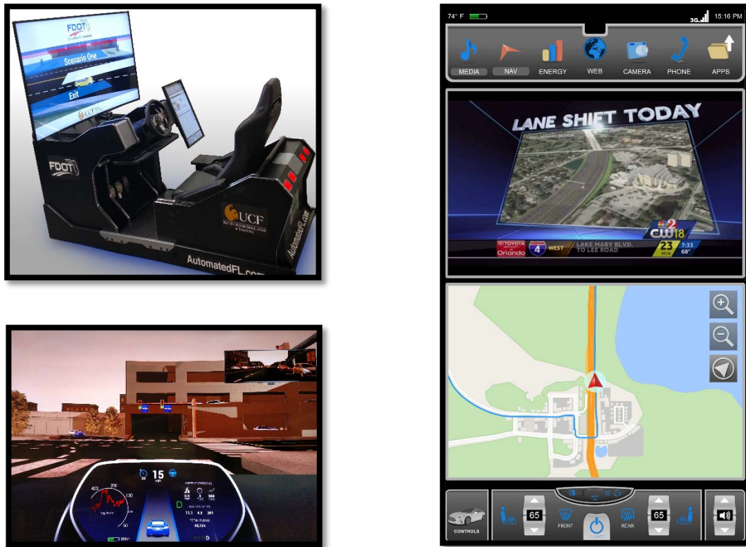
Figure 11: The FDOT DCVS is an advanced simulator used for measuring human experiences with connected vehicles. Top Left: A side view of the complete simulator system. Right: The complete interactive dashboard console display showing the routing and media player panes. Bottom-left: A view from the main screen of the simulator as the car approaches a parking garage. The dashboard iconography replicates (with permission) that of the Tesla Model S.
