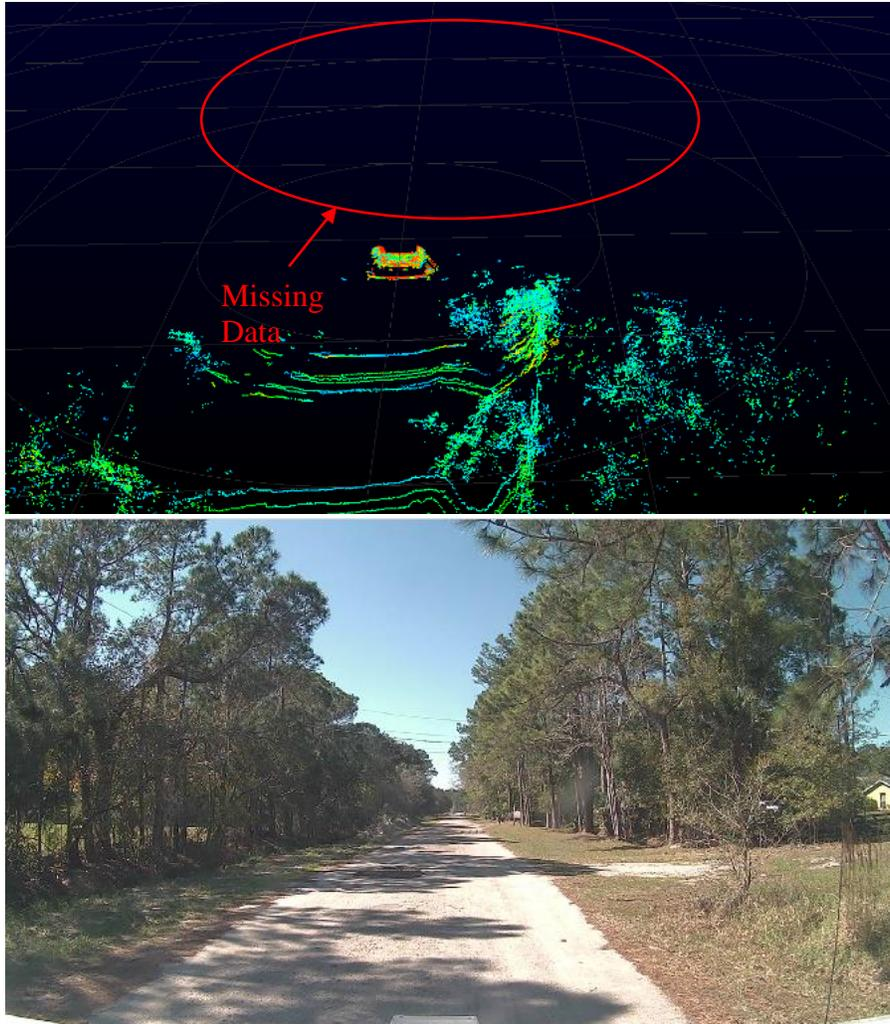
**Figure 20: Data loss shown in the LIDAR playback**
