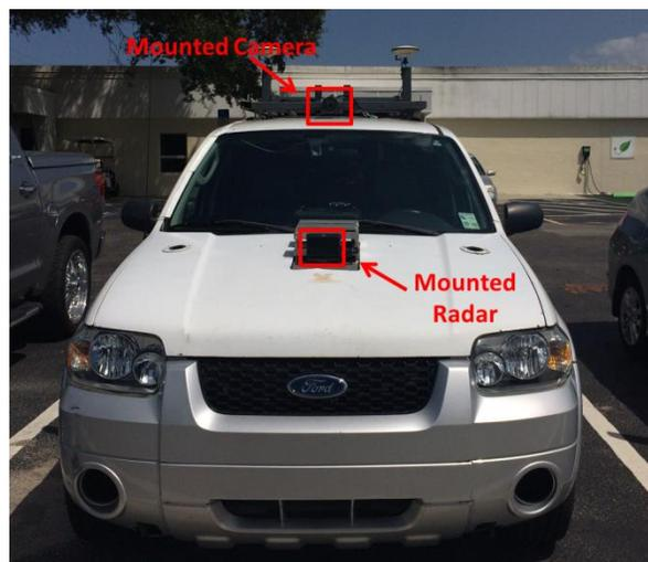
**Figure 4: Samsung Camera and Continental Radar as mounted on the Plan B vehicle.**
