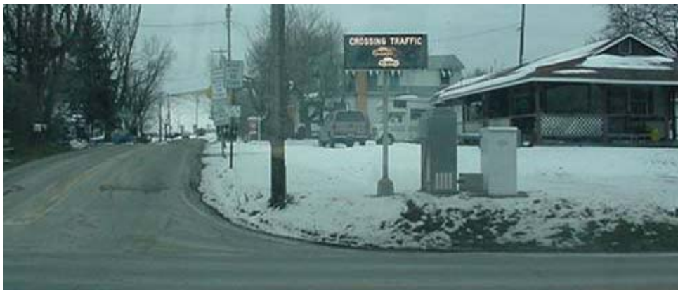
Figure 20 PennDOT CAS Minor Road Display of Approaching Major Road Vehicles
