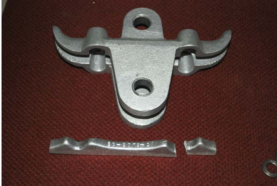
Figure 6-6. Span wire clamp with broken piece (Photo courtesy of author)
