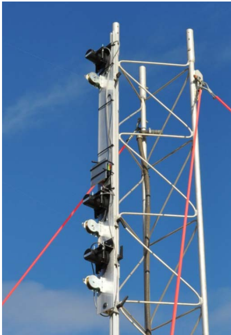
Figure 3-10. Mounting system for string potentiometers (Photos courtesy of author)
