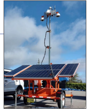
The Smart Work Zone Trailer, seen here before its initial deployment, combines several technologies, including a collapsible solar array and three video cameras atop the trailer.
