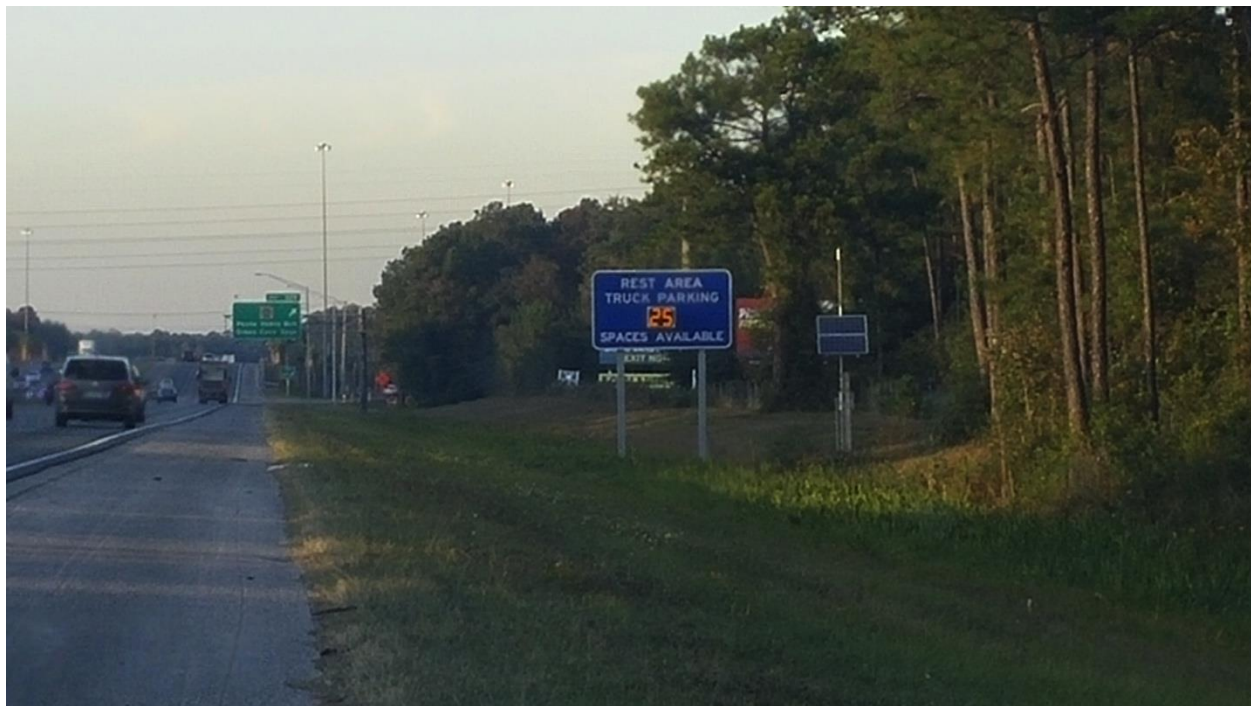
Figure 4.4 – Truck Parking Availability Embedded DMS Module
